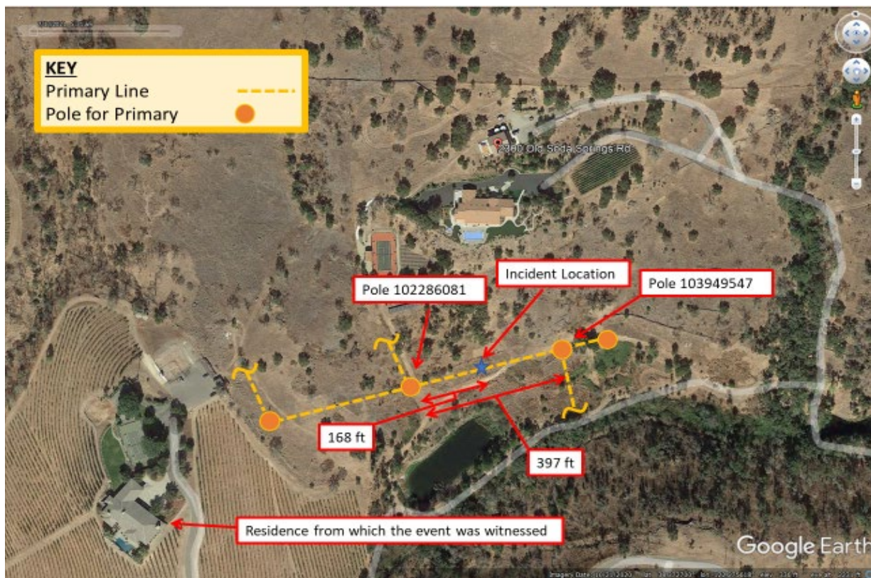
Figure 1: Sketch of Incident Location. Primary Line refers to the Subject Circuit conductors.
