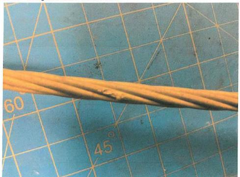
Photo No. 14: Arcing evidence on the conductor
