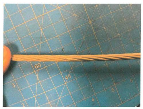
Photo No. 11: Arcing evidence on the conductor
