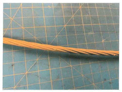
Photo No. 21: Arcing evidence on the conductor
