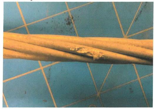
Photo No. 12: Arcing evidence on the conductor
