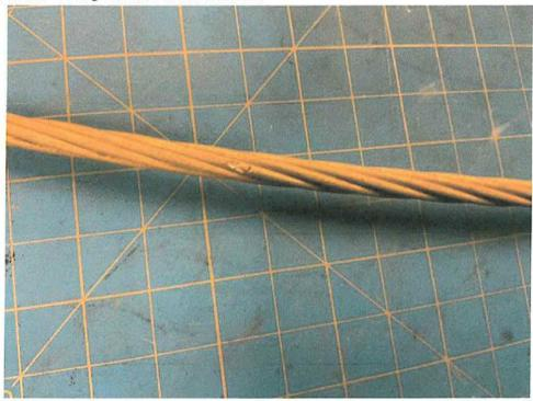
Photo No. 20: Arcing evidence on the conductor
