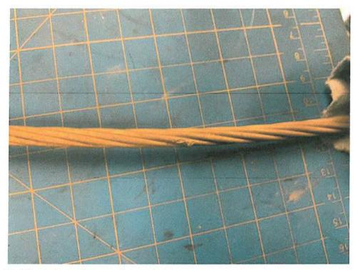
Photo No. 19: Arcing evidence on the conductor
