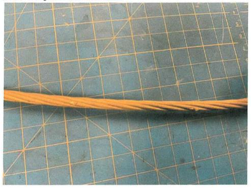
Photo No. 18: Arcing evidence on the conductor
