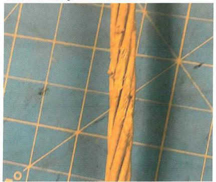
Photo No. 6: Arcing evidence on the conductor
