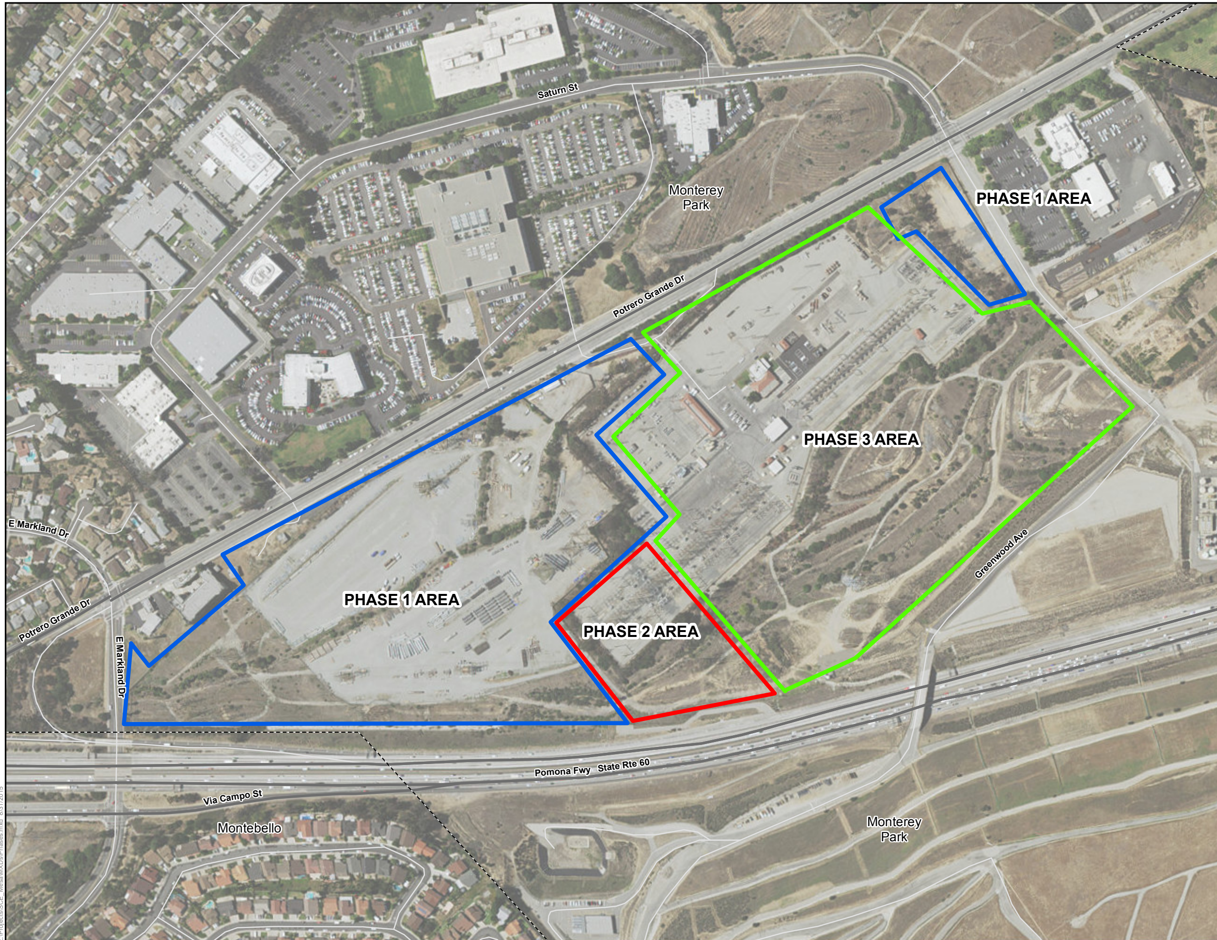
Figure 3: Grading Phase Areas Mesa 500 kV Substation Project
