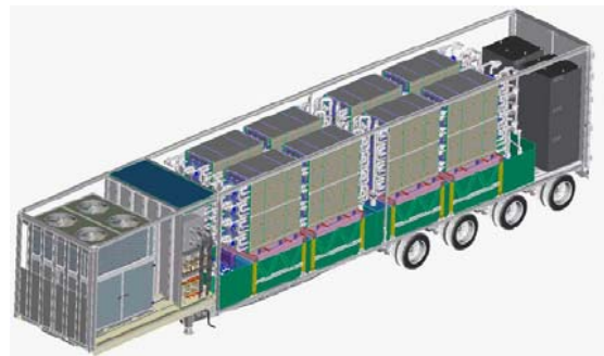
Zinc Bromine Flow Batteries
