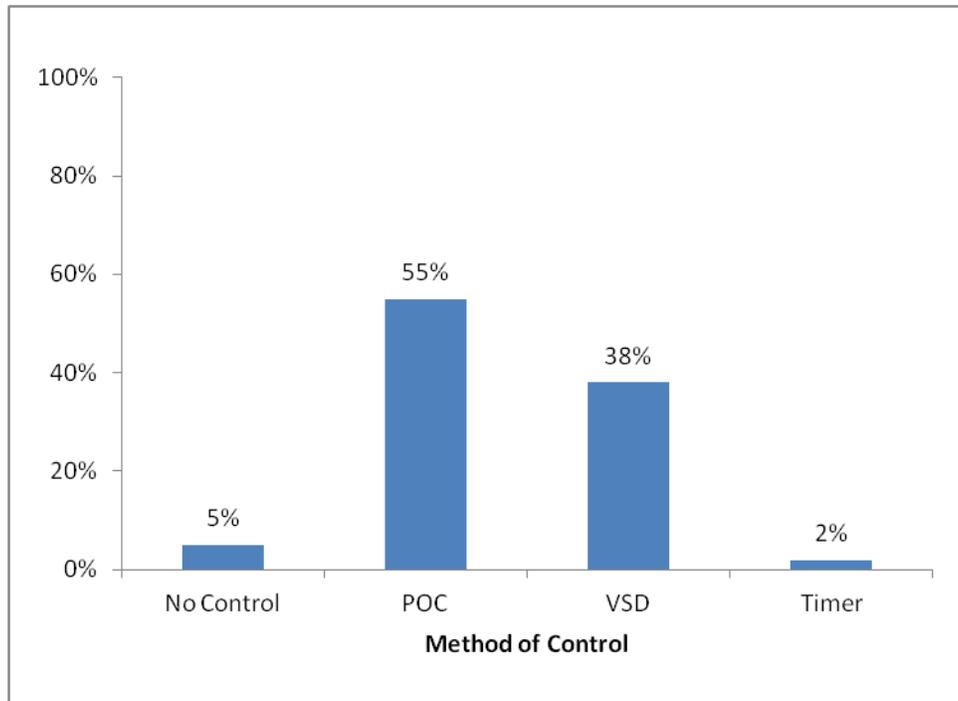
**Table 9: Manufacturers' Estimated Distribution of Control Methods for Rod Beam Pumps at Major Oil Producers**
