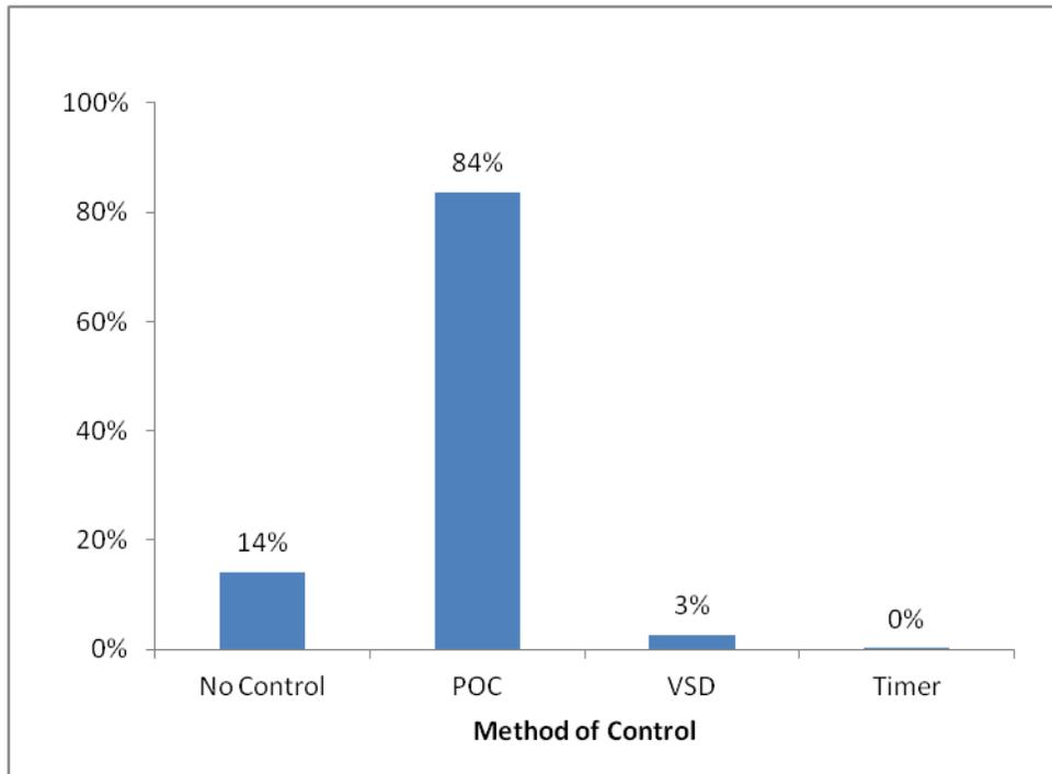
**Table 3: Distribution of Control Methods for Rod Beam Pumping at Major Oil Producers**
