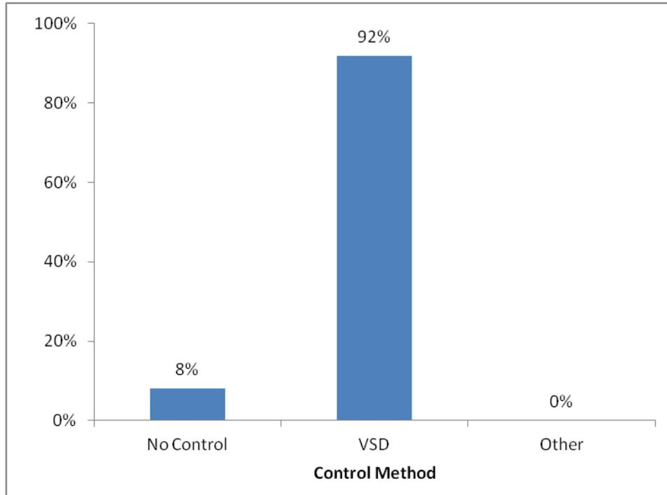
**Table 8: Distribution of Control Methods for PCP Operation at Minor Oil Producers**
