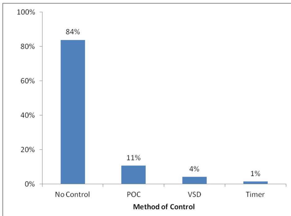
**Table 6: Distribution of Control Methods for Rod Beam Pumping at Minor Oil Producers**
