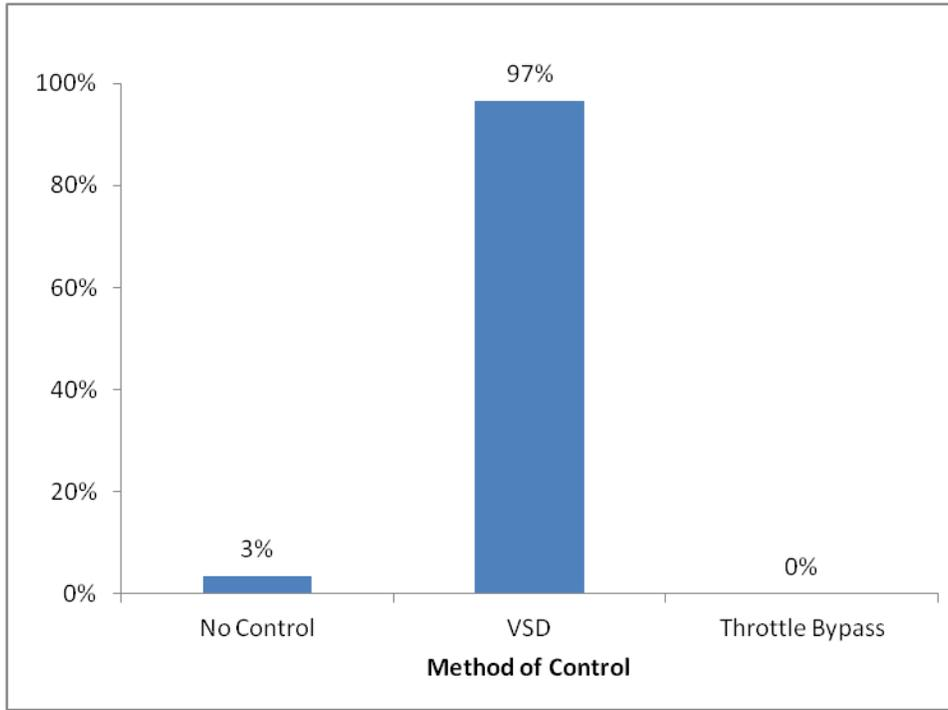
**Table 7: Distribution of Control Methods for ESP Operation at Minor Oil Producers**
