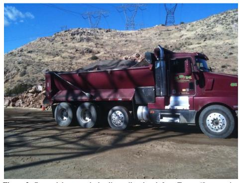
**Figure 2:** Covered dump trucks hauling soil and rock from Tower 68 excavation to Lancaster landfill, Segment 5.
