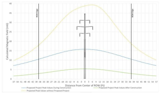
Figure 82 – Typical Magnetic Field Levels for Segment 1 Section 4 Structure 683 – Structure 912, Str. 707-708 at 200 Amps
