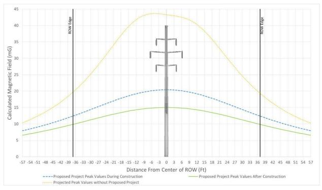
Figure 4 - Typical Magnetic Field Levels for Segment 1 Section 2 Structure 214 – Structure 442, Str. 251 - 252 at 200 Amps
