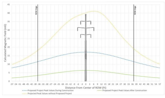
Figure 10 - Typical Magnetic Field Levels for Segment 1 Section 5 Structure 912 – Inyokern Substion, Str. 957 - 958 at 200 Amps
