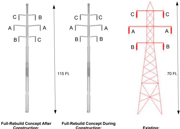
Construction: Double Circuit – Monopole Figure not to Scale Full-Rebuild Concept During Construction: Double Circuit – Monopole Figure not to Scale
