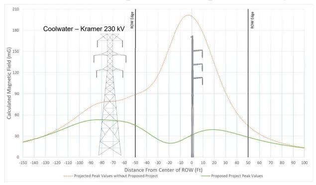
Assuming Drake ACSR conductor, Top-Bottom phasing 0°,120°,240°-0°,120°,240°, and 400 Amps for parallel line.
