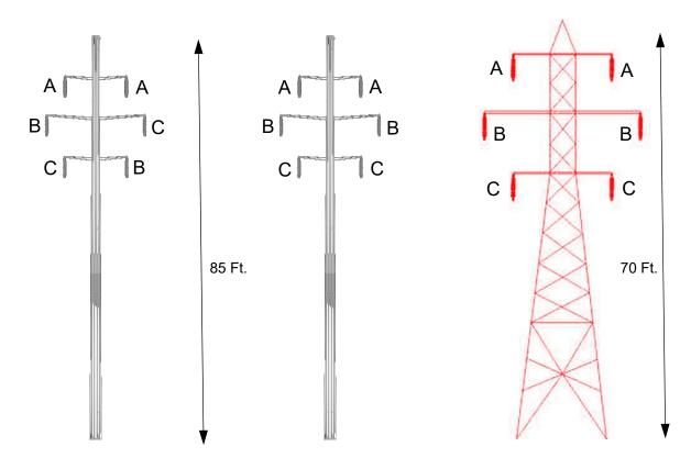
Full-Rebuild Concept After Construction: Double Circuit – Monopole Figure not to Scale Full-Rebuild Concept During Construction: Double Circuit – Monopole Figure not to Scale
