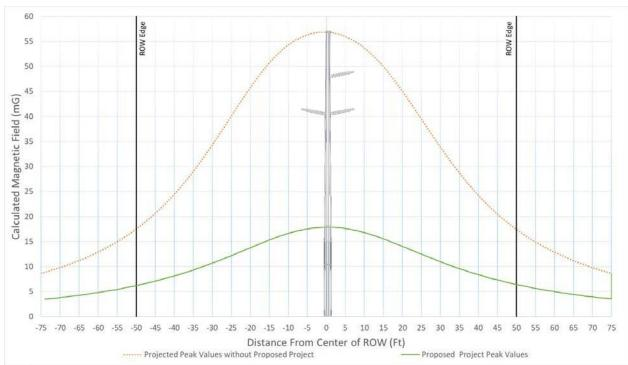
Figure 42 - Typical Magnetic Field Levels for Segment 4 Section 9 Structure 128753 – Structure 128774, Str. 128770 - 128771 at 270 Amps
