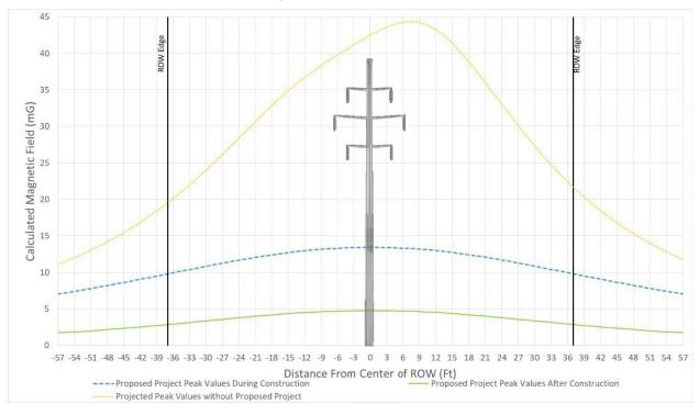
Figure 84 – Typical Magnetic Field Levels for Segment 1 Section 5 Structure 912 – Inyokern Substation, Str. 1045-1046 at 200 Amps
