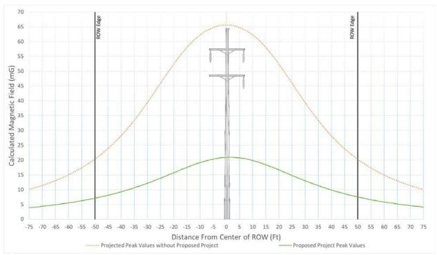
Figure 60 - Typical Magnetic Field Levels for Segment 4 Section 18 Structure 1281015 – Structure 1281039, Str. 1281018 - 1281019 at 315 Amps
