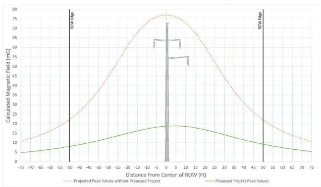
Figure 72 - Typical Magnetic Field Levels for Segment 4 Section 24 Mountain Pass Substation – Structure 1281210, Str. 1281198 - 1281199 at 330 Amps
