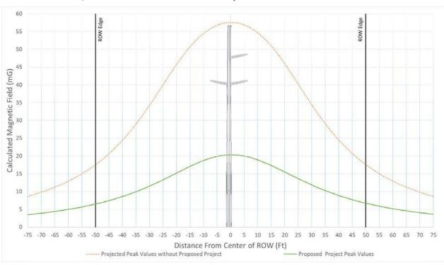
Figure 48 - Typical Magnetic Field Levels for Segment 4 Section 12 Structure 128840 – Structure 128882, Str. 128867 - 128868 at 270 Amps
