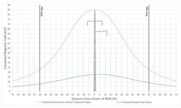
Figure 74 - Typical Magnetic Field Levels for Segment 4 Section 25 Structure 1281210 - Ivanpah Substation, Str. 1281210 - 1281211 at 330 Amps
