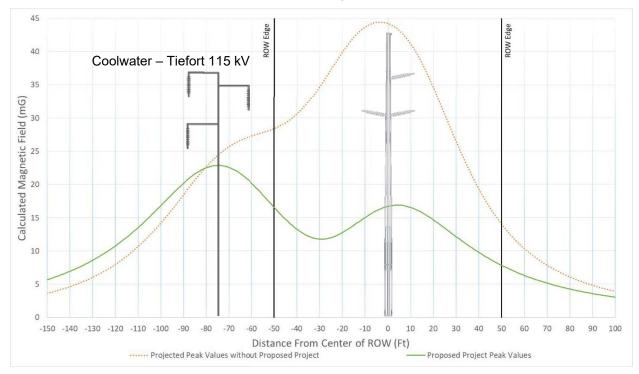
Assuming Partridge ACSR conductor, Top-Bottom phasing 0°,120°,240° and 400 Amps for parallel line. Graph is extended to show the influence of the parallel line.
