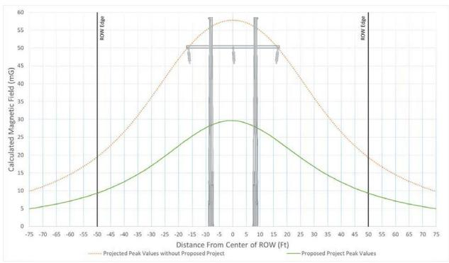
Figure 54 - Typical Magnetic Field Levels for Segment 4 Section 15 Baker Substation – Structure 128949, Str. 128939 - 128940 at 315 Amps
