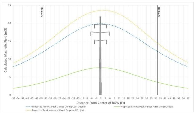
Figure 8 - Typical Magnetic Field Levels for Segment 1 Section 4 Structure 683 – Structure 912, Str. 768 - 769 at 200 Amps
