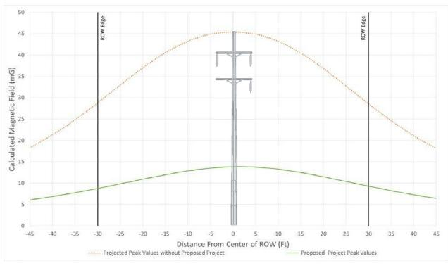
Figure 30 - Typical Magnetic Field Levels for Segment 4 Section 3 Structure 128595 – Structure 128638, Str. 128614-128615 at 260 Amps
