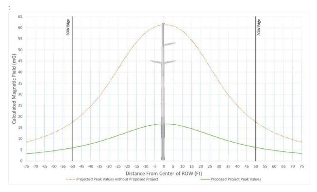
Figure 96 – Typical Magnetic Field Levels for Segment 4 Section 2 Structure 128595 – Structure 128638, Str. 128608 – 128609 at 260 Amps
