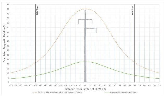
Figure 68 - Typical Magnetic Field Levels for Segment 4 Section 22 Structure 1281146 – Structure 1281167, Str. 1281154 – 1281155 at 315 Amps
