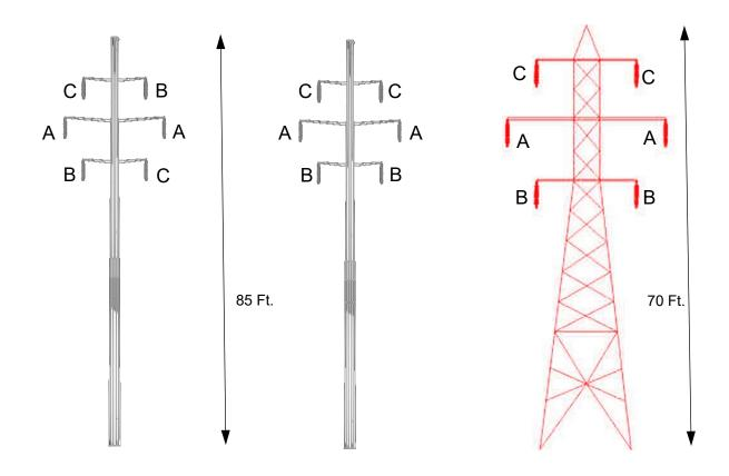
Full-Rebuild Concept After Construction: Double Circuit – Monopole Figure not to Scale Full-Rebuild Concept During Construction: Double Circuit – Monopole Figure not to Scale
