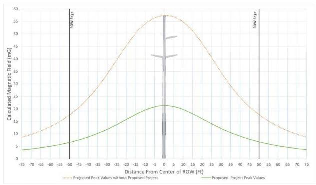
Figure 50 - Typical Magnetic Field Levels for Segment 4 Section 13 Structure 128882 – Structure 128904, Str. 128885 - 128886 at 270 Amps
