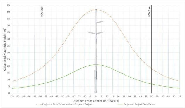
Figure 46 - Typical Magnetic Field Levels for Segment 4 Section 11 Structure 128817 – Structure 128840, Str. 128825 - 128826 at 270 Amps
