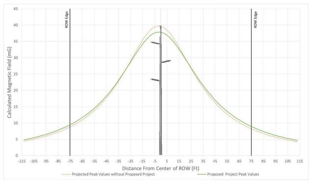
Figure 24 - Typical Magnetic Field Levels for Segment 3S Section 2 Tortilla Substation – Coolwater Substation, Str. 1811388E - 1811383E at 600 Amps
