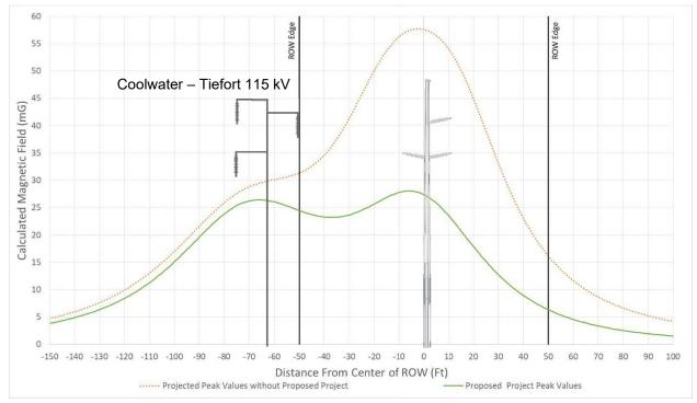
Assuming Partridge ACSR conductor, Top-Bottom phasing  $0^{\circ}$ ,120 $^{\circ}$ ,240 $^{\circ}$  and 400 Amps for parallel line. Graph is extended to show the influence of the parallel line.
