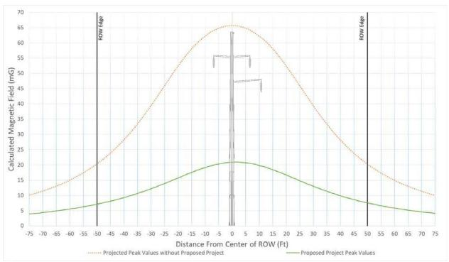
Figure 62 - Typical Magnetic Field Levels for Segment 4 Section 19 Structure 1281039 – Structure 1281082, Str. 1281067 - 1281068 at 315 Amps
