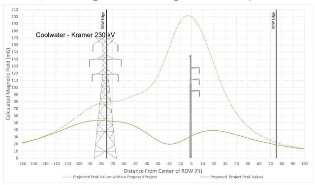
Figure 20 - Typical Magnetic Field Levels for Segment 3N Kramer Substation – Coolwater Substation, Str. N1561186E\_S1561185E- N4457229E\_S4457230E at 860 Amps
