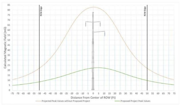
Figure 64 - Typical Magnetic Field Levels for Segment 4 Section 20 Structure 1281082 – Structure 1281104, Str. 1281098 - 1281099 at 315 Amps
