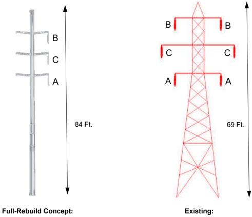
Full-Rebuild Concept: Single Circuit – Monopole Figure not to Scale
