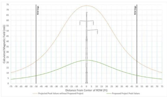
Figure 66 - Typical Magnetic Field Levels for Segment 4 Section 21 Structure 1281104 – Structure 1281146, Str. 1281145 - 1281146 at 315 Amps
