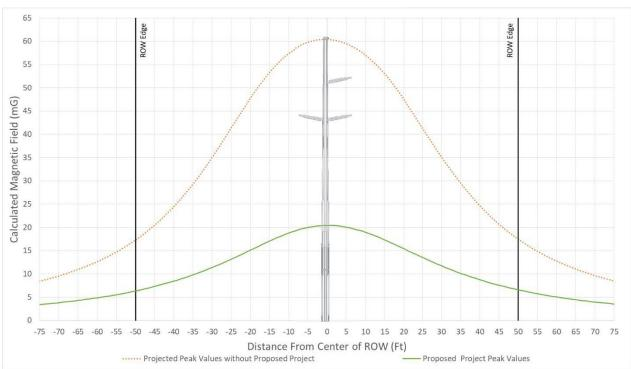
Figure 34 - Typical Magnetic Field Levels for Segment 4 Section 5 Structure 128660 – Structure 128699, Str. 128684 - 128685 at 260 Amps
