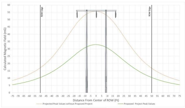
Figure 28 - Typical Magnetic Field Levels for Segment 4 Section 2 Structure 128574 – Structure 128595, Str. 128585 - 128586 at 260 Amps
