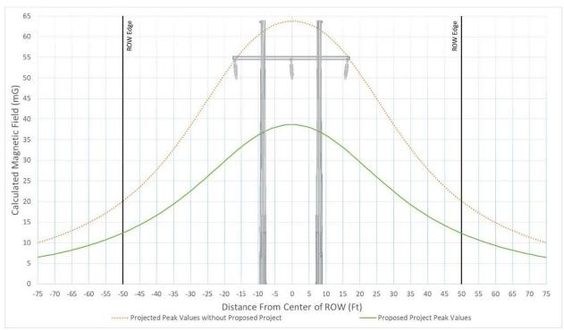
Figure 58 - Typical Magnetic Field Levels for Segment 4 Section 17 Structure 128971 – Structure 1281015, Str. 128990 - 128991 at 315 Amps
