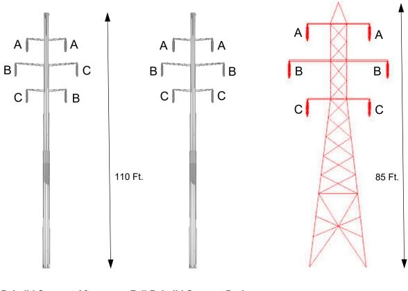
Full-Rebuild Concept After Construction: Double Circuit – Monopole Figure not to Scale Full-Rebuild Concept During Construction: Double Circuit – Monopole Figure not to Scale
