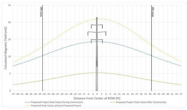
Figure 6 - Typical Magnetic Field Levels for Segment 1 Section 3 Structure 442 – Structure 683, Str. 544 - 545 at 200 Amps
