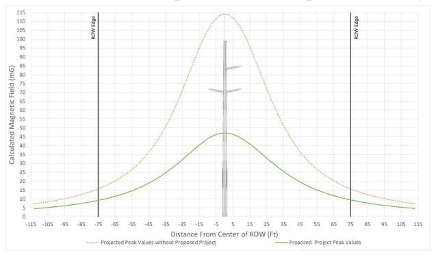
Figure 22 - Typical Magnetic Field Levels for Segment 3S Section 1 Kramer Substation – Tortilla Substation, Str. NA560144AE\_SA560144BE - NA560143AE\_SA560143BE at 725 Amps
