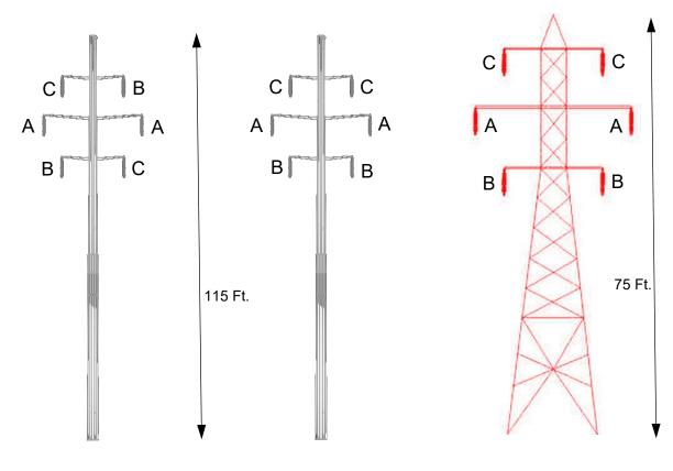
Full-Rebuild Concept During Construction: Double Circuit – Monopole Figure not to Scale
