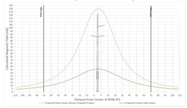
Figure 90 – Typical Magnetic Field Levels for Segment 3S Section 1 Kramer Substation – Tortilla Substation, Str. NA560091SE\_SA560091BE – NA560090AE\_SA560090BE at 725 Amps
