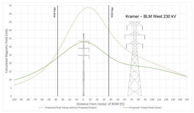
Figure 16 - Typical Magnetic Field Levels for Segment 2 Section 3 Randsburg Substation – Structure 121042, Str. 121124 - 121123 at 840 Amps
