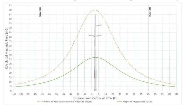
Figure 92 – Typical Magnetic Field Levels for Segment 3S Section 1 Kramer Substation – Tortilla Substation, Str. NA560113AE\_SA560113BE – NA560112AE\_SA560112BE at 725 Amps
