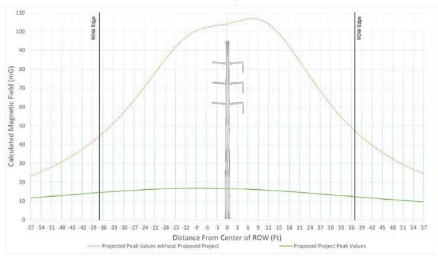
Figure 86 – Typical Magnetic Field Levels for Segment 2 Section 1 Kramer Substion – Structure 121255, Str. 121165 – 121166 at 840 Amps
