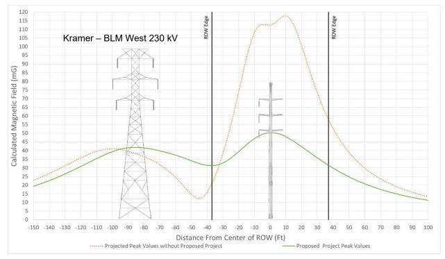
Assuming Curlew ACSR conductor, Top-Bottom phasing 0°,120°,240°-0°,120°,240°, and 400 Amps for parallel line.
