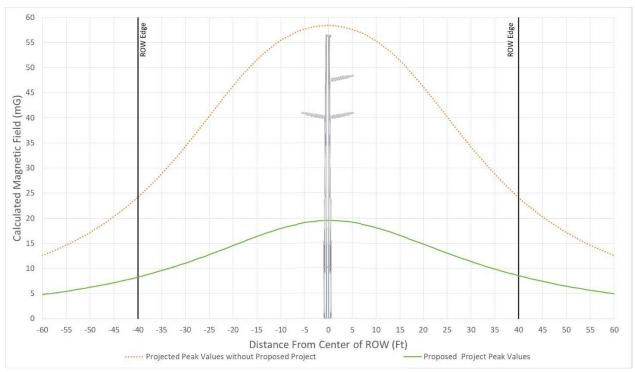
Figure 32 - Typical Magnetic Field Levels for Segment 4 Section 4 Structure 128638 – Structure 128660, Str. 128645 - 128646 at 260 Amps
