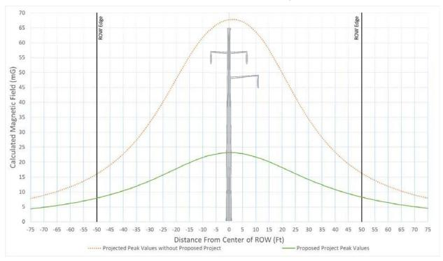
Figure 70 - Typical Magnetic Field Levels for Segment 4 Section 23 Structure 1281167 – Mountain Pass Substation, Str. 1281175 - 1281176 at 315 Amps
