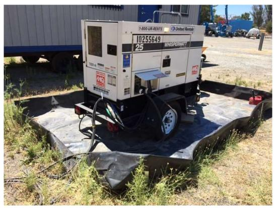
Figure 4 – Secondary containment pushed down by electrical cords – view southwest, July 21, 2017.
