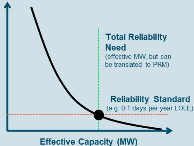
*LOLP modeling provides Total Reliability Need in effective capacity MW to meet <0.1 days/yr LOLE, can be converted to a PRM*
