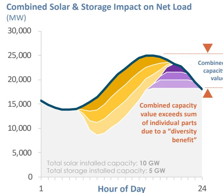
The ELCC approach inherently captures both capacity & energy adequacy
