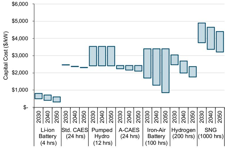
Figure 4-1: Installed Capital Cost of Energy Storage Technologies (2022 \$/kW)
