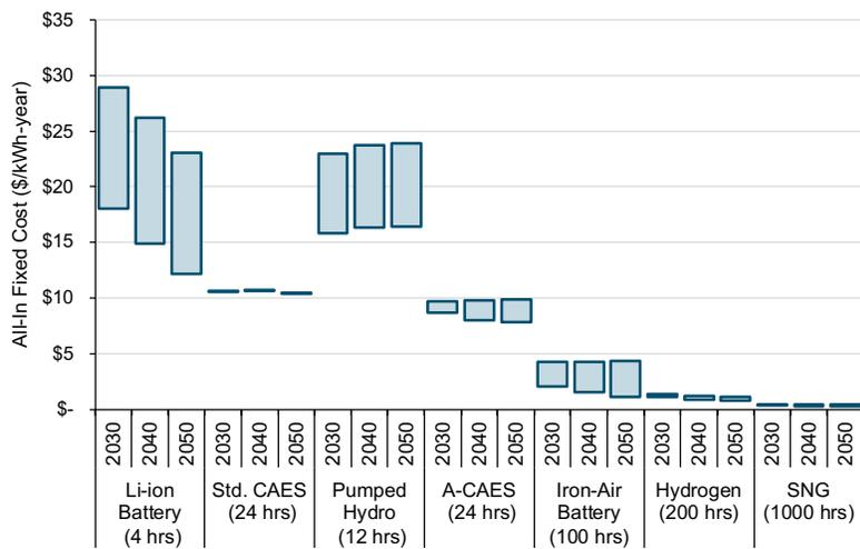
**Figure 4-4: Levelized All-In Fixed Cost of Storage Technologies Specified Storage Duration, Normalized by Storage Duration (2022 \$/kWh-yr)**
