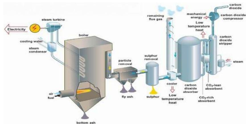
A key advantage of post-combustion CCS is that it offers an option for existing power plants to mitigate emissions through retrofitting, presenting an option to repurpose existing natural gas infrastructure. In addition, CO<sub>2</sub> in flue gas is
