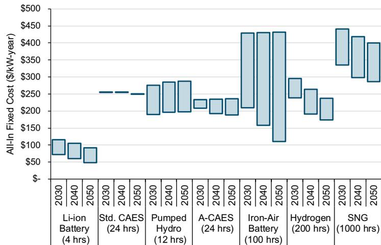
**Figure 4-3: Levelized All-In Fixed Cost of Storage Technologies at Specified Duration (2022 \$/kW-yr)**
