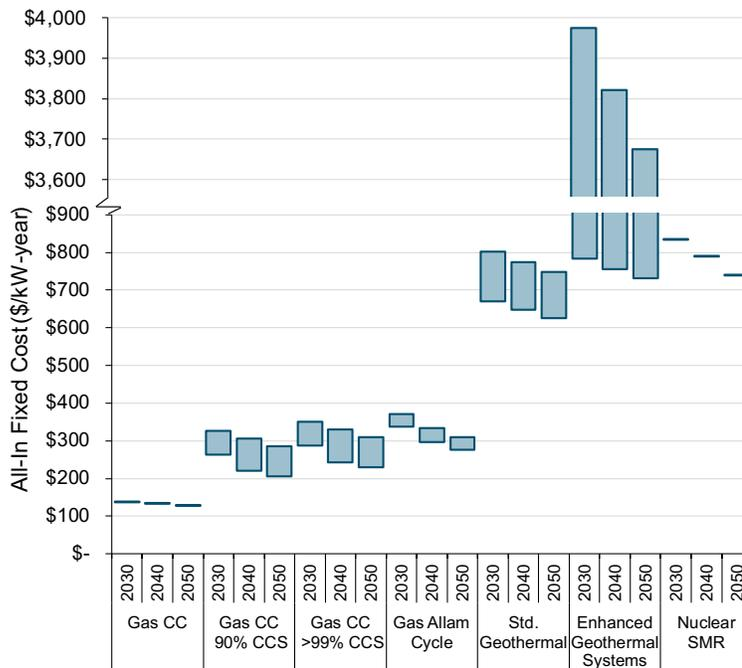
**Figure 4-7: Levelized Fixed Costs of Generation Resource (2022 \$/kW-yr)**
