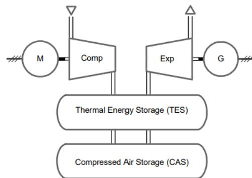
Generally, the advantage of A-CAES is that it could provide emissions-free, long-duration operation with reasonably high round trip efficiency. The primary disadvantage of A-CAES is that it requires specific underground geologic formations to work, which may not be ideal points for grid interconnection. Additionally, A-CAES is a relatively immature technology.
