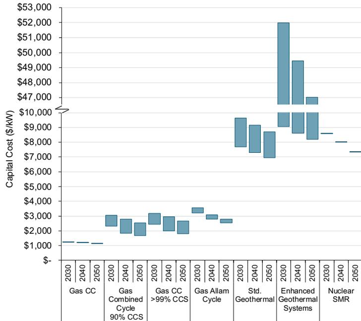
Figure 4-5: Installed Capital Costs of Generation Resources (2022 \$/kW)
