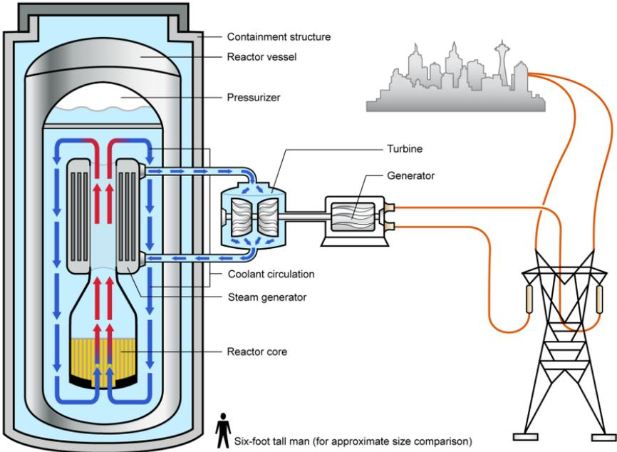
advantage of the smaller, modular design is increased flexibility in construction: individual units can be manufactured in a factory and aggregated at a power plant site incrementally as needed. This may allow for quicker technology learning and standardization through more iterations of building a standardized design, potentially resulting in shorter construction and permitting times. Shorter lead
