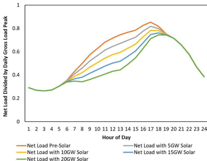
The orange line in Figure 1. Illustrative Net Load Shift Due to Solar Penetration depicts the net load assuming no solar (i.e., gross load less other modifiers such as wind, energy efficiency, etc.), and the different colored lines below the no solar line depict net loads at various penetrations of solar. The figure clearly depicts a time shift in the “net load peak” of the system. As the new net load peak approaches
