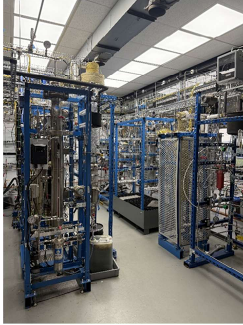
Figure 2 Laboratory test rigs - Bench scale gasification and methanation units at GTI Energy
