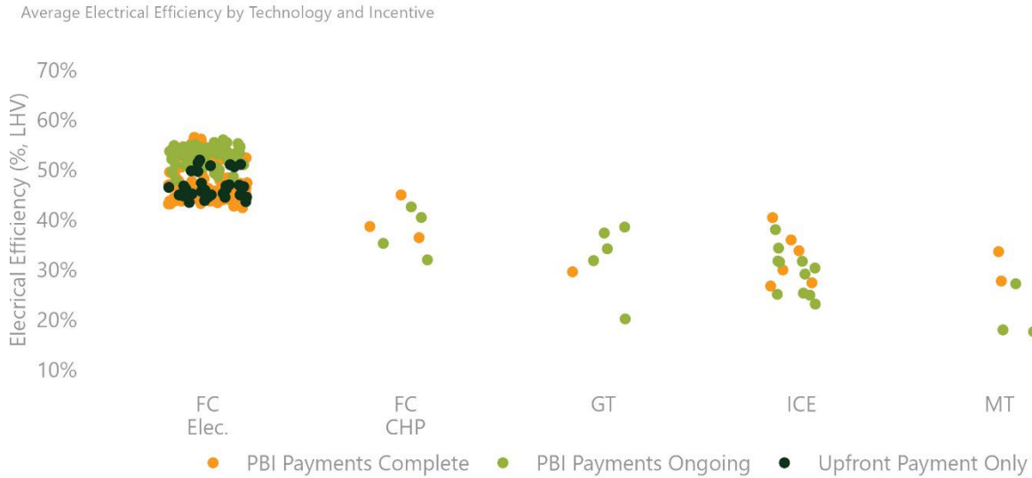
FIGURE C-29: DISTRIBUTION OF OBSERVED 2021 ELECTRICAL EFFICIENCIES BY GENERATION TECHNOLOGY AND INCENTIVE
