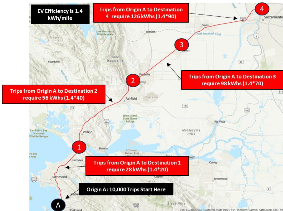
Figure C-4. Cumulative Energy Step 4 Example: Determine Trip BEV Energy Requirement
