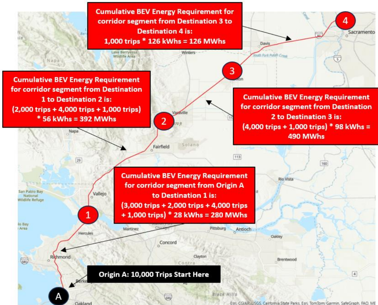
Figure C-5. Cumulative Energy Step 5 Example: Determine Cumulative BEV Energy Value
