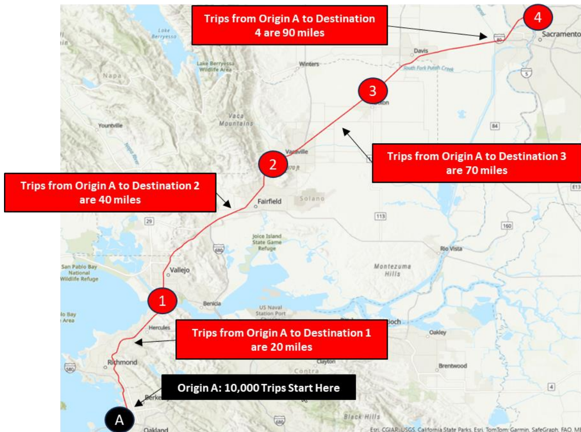
Figure C-3. Cumulative Energy Step 3 Example: Determine Length of Trip
