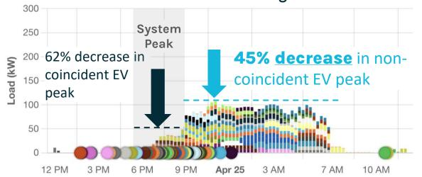
Load Balancing **flattens EV load** in off-peak to resolve timer and noncoincident peaks
