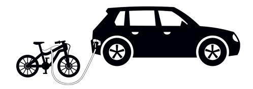
V2L adapter for EVPE: generic power output for cord connected loads
