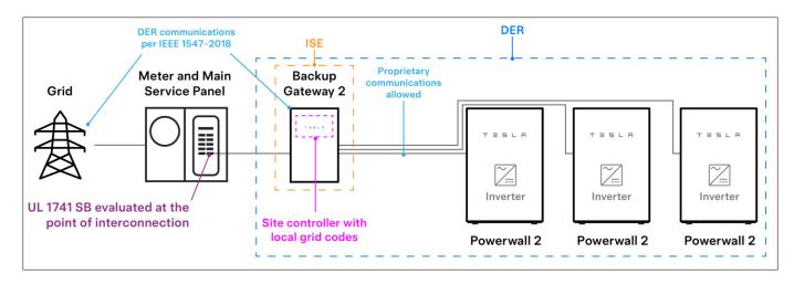
Figure 2: Tesla Powerwall 2 grid performance diagram
