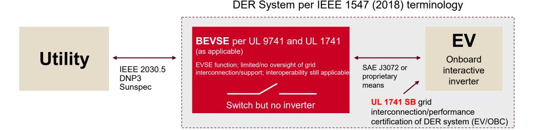
Nationally Recognized Testing Laboratory (NRTL) Electric vehicle power export (EVPE) Interconnection systems equipment (ISE) Onboard charger (OBC) Bidirectional electrical vehicle supply equipment (BEVSE)
