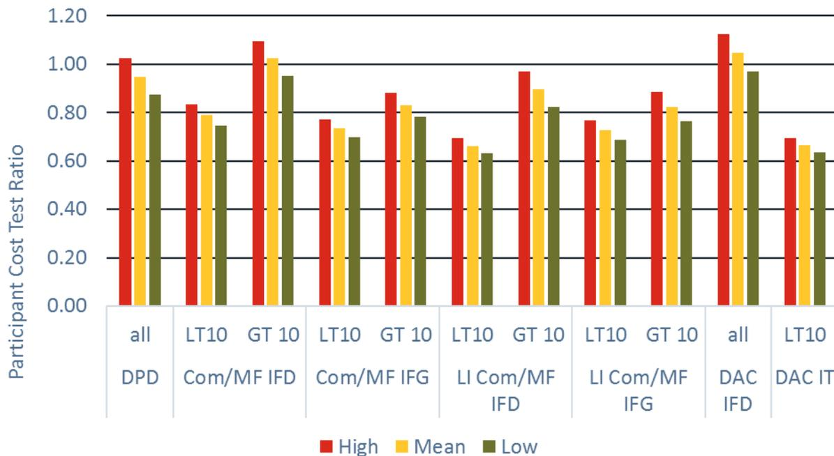
The findings presented in Figure 4-10 illustrate that IFD systems larger than 10 kW<sub>th</sub> drive the higher PCT values presented in Figure 4-8. Systems with less than 10 kW<sub>th</sub> of capacity have a substantially higher cost per therm savings and substantially smaller anticipated therm and bill savings, leading the smaller IFD systems to have a lower PCT than the larger systems. This may be evidence of economies of scale for larger systems.
