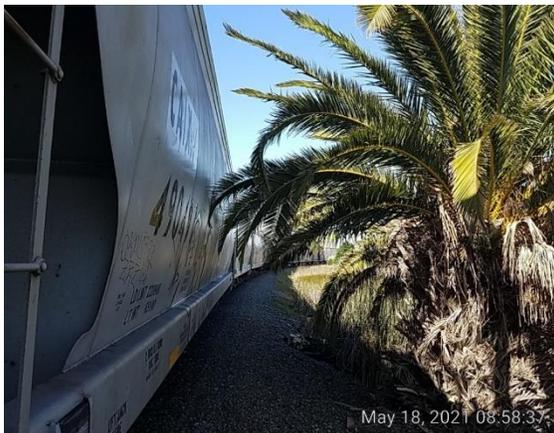
Before: North side of track 3040 – Tree branches are contacting the equipment.
