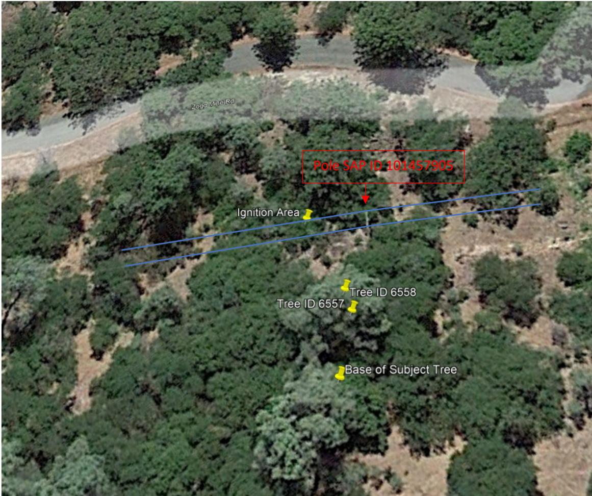
**Figure 1:** Diagram of the Base of the Subject Tree, Tree ID 6557, Tree ID 6558, Ignition Area, and PG&E Facilities.<sup>25</sup> The lines marked in blue show approximate conductor path and continue east and west in both directions. The pinned locations of Tree IDs 6557 and 6558 are based on GPS coordinates from PG&E VM records. The location of the Subject Tree is based on CalFire's GPS records. All locations represent the approximate locations of the base of the
