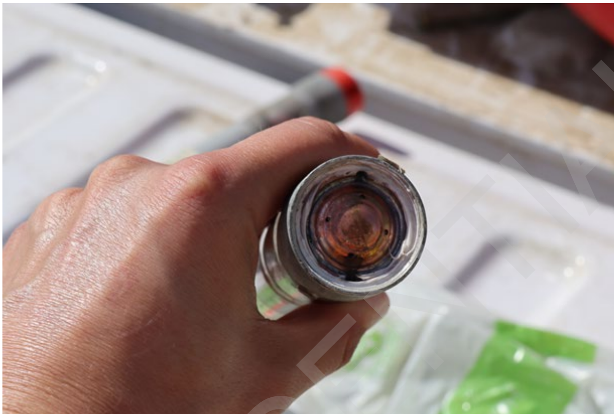
Figure 11: The East phase fuse is missing the red cap, indicating that the fuse activated and opened the circuit.
