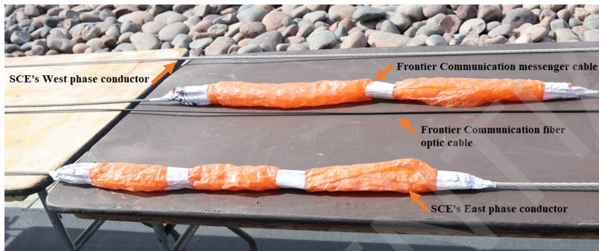
Figure 16: SCE's East and West phase conductors and Frontier Communications' fiber optic cable and messenger cable.
