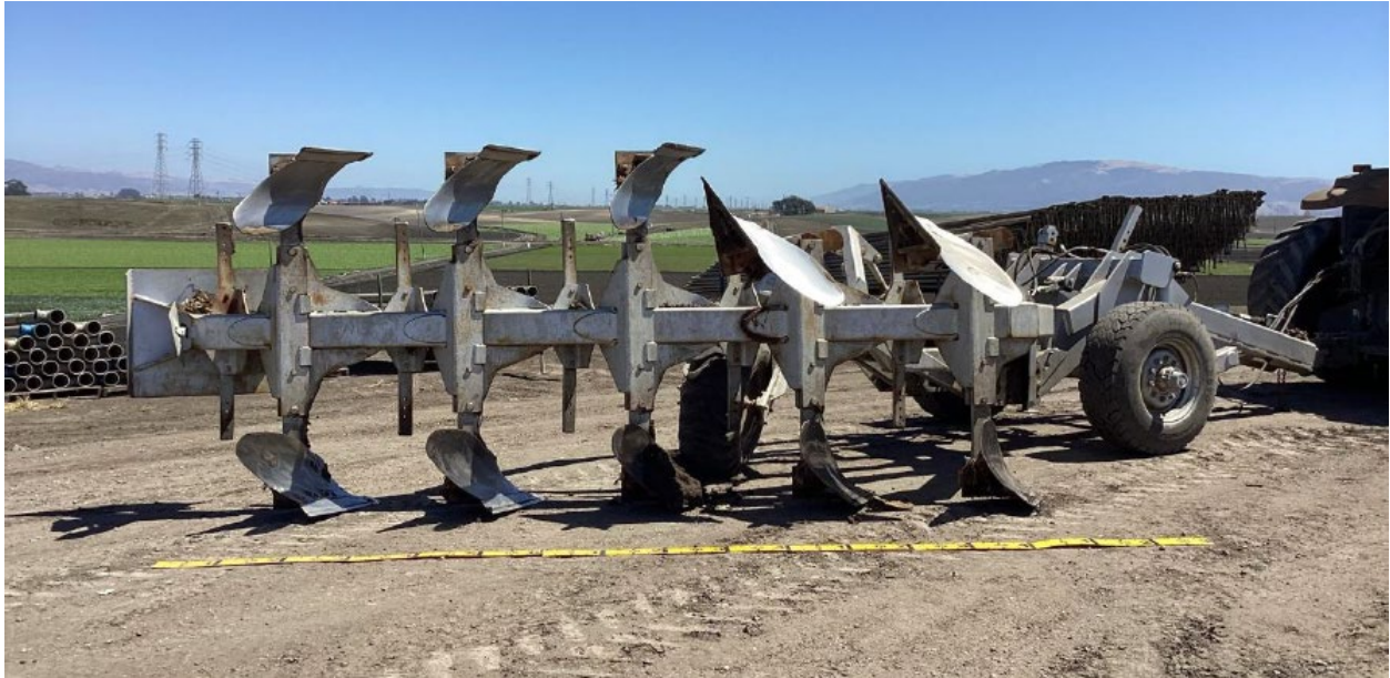
Figure 3. Photo of the ripper that struck the pipe.
