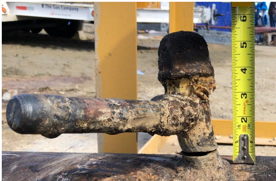
Figure 3. Damaged 1-inch stub “abandoned service tee”
