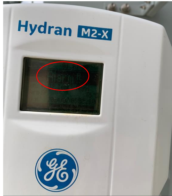
Figure 3: GSU Transformer T1 Hydran M2-X gas monitoring system with an active alarm.
