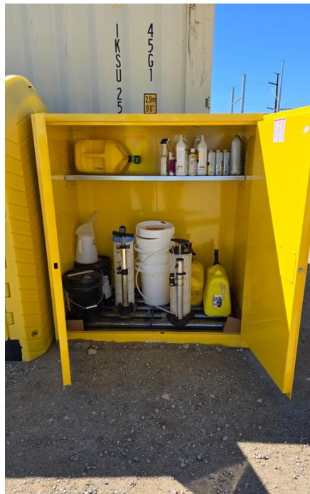
Figure 4: Flammable material storage cabinet without a self-closing mechanism.
