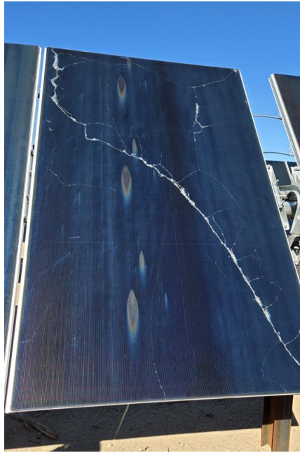
Figure 7: Damaged solar PV panel.
