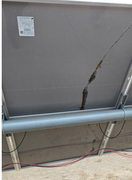
Figure 5: Damaged solar PV panel.
