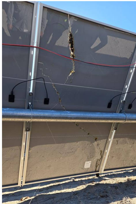
Figure 6: Damaged solar PV panel.
