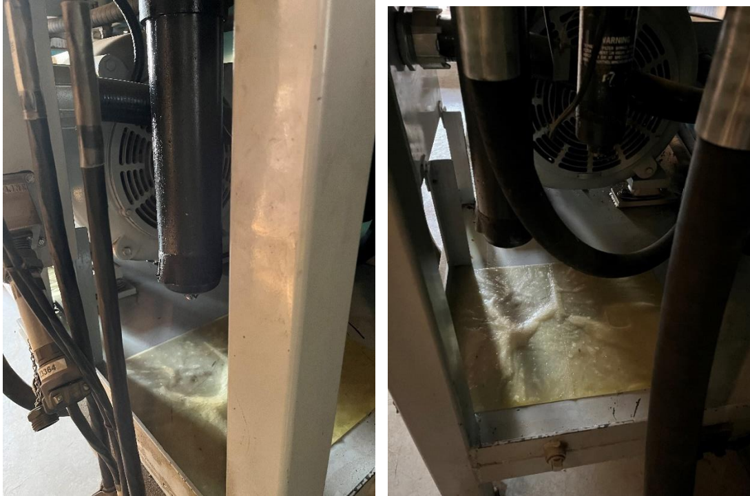
Figure 18: Saturated absorbent padding under hydraulic filters.
