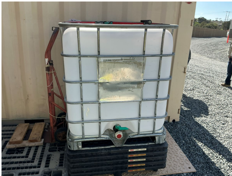
Figure 13: An IBC tote without a label indicating its contents.
