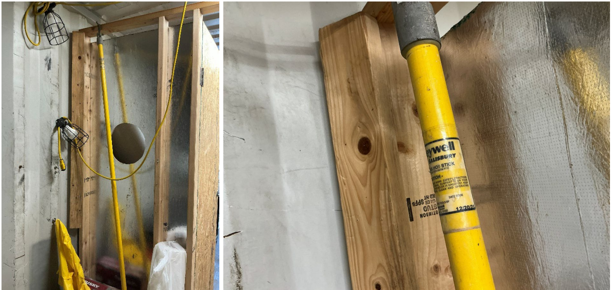
Figure 4: Hot stick with 2021 calibration tags found in Valley Center Storage container.
