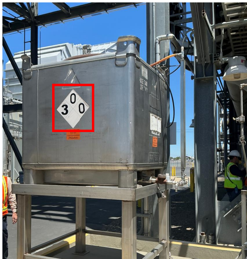
Figure 15: Color-faded on NFPA 704 Placard.
