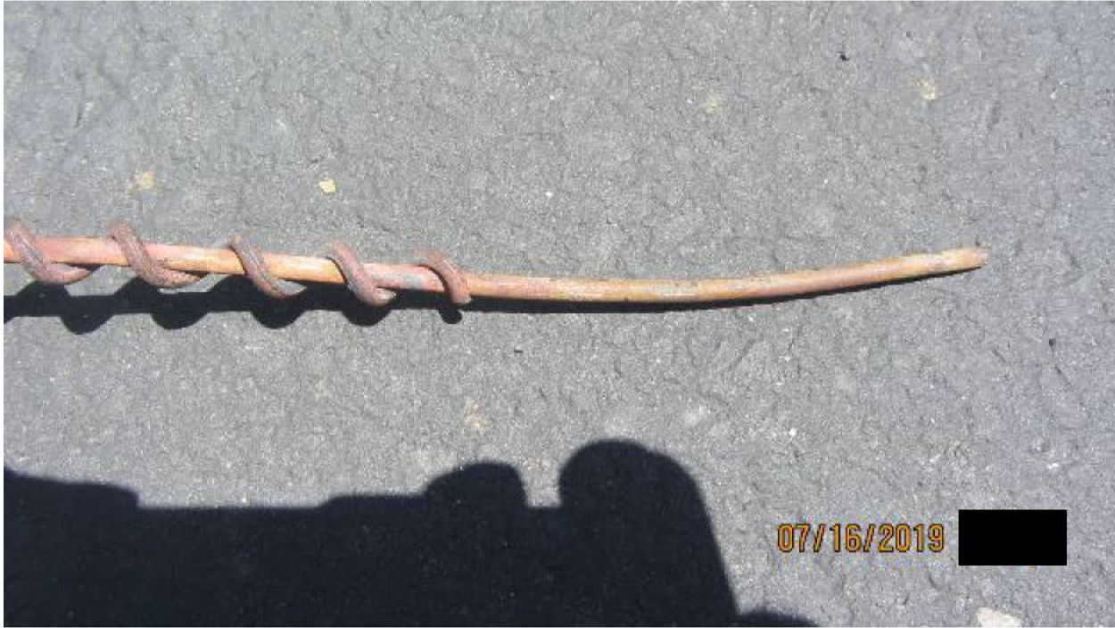
Figure 11: Conductor 2 and the portion of tie wire still attached.
