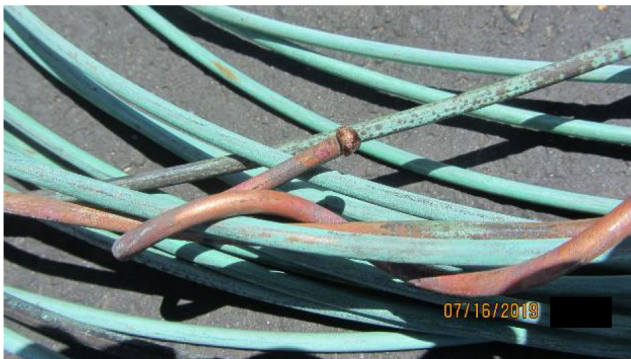
Figure 10: Melted end of Conductor 1.
