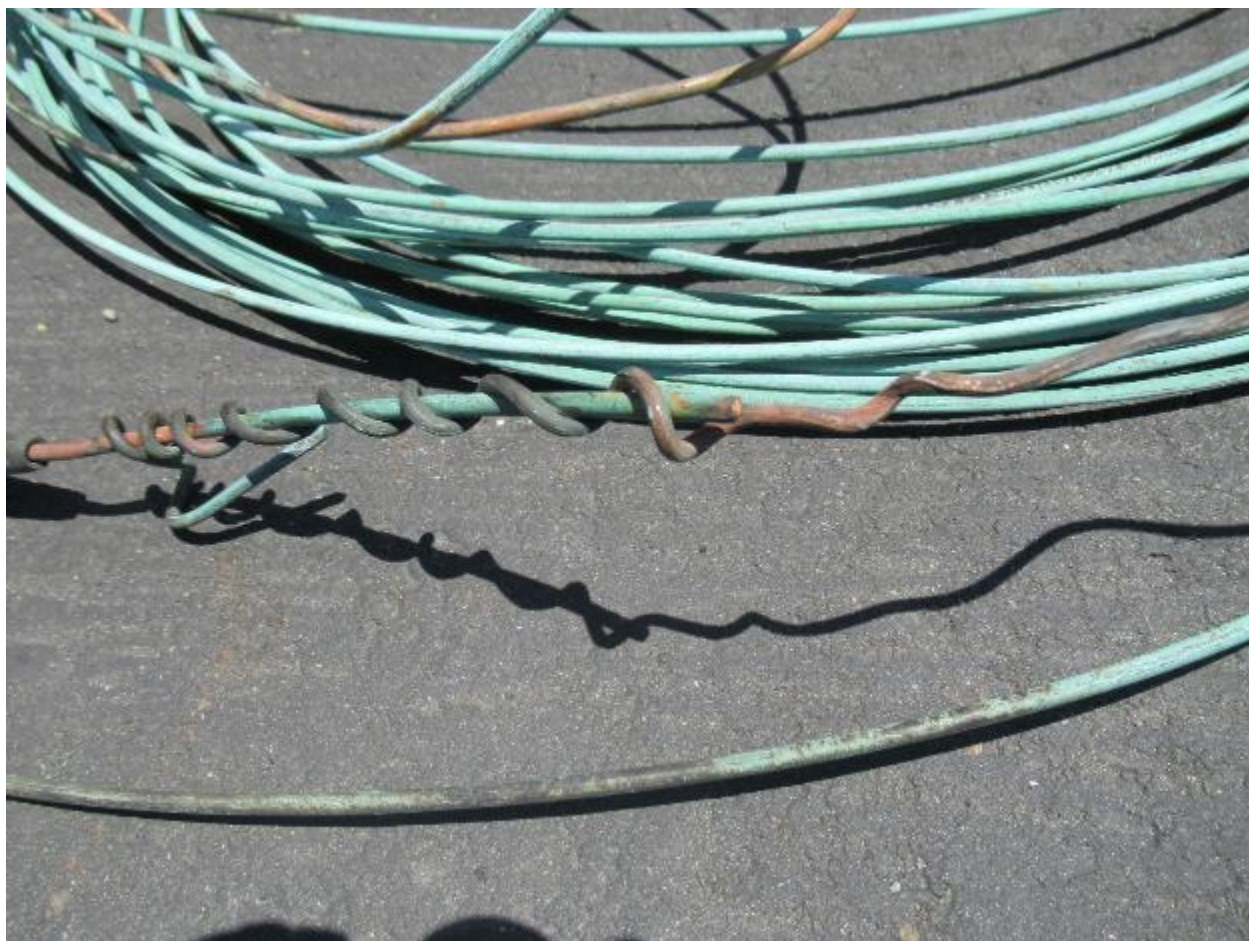
Figure 8: Conductor 1, with a portion of a tie wire still wrapped around one end.
