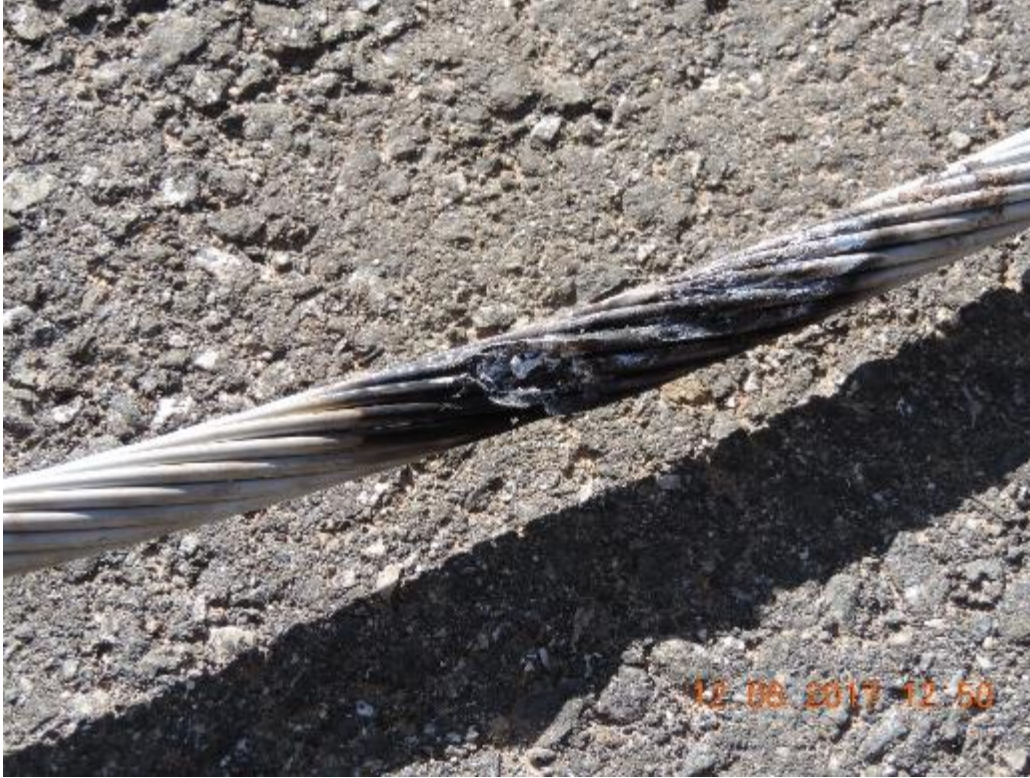
Figure 12: Loss of material on a jumper wire from pole 4389254E.
