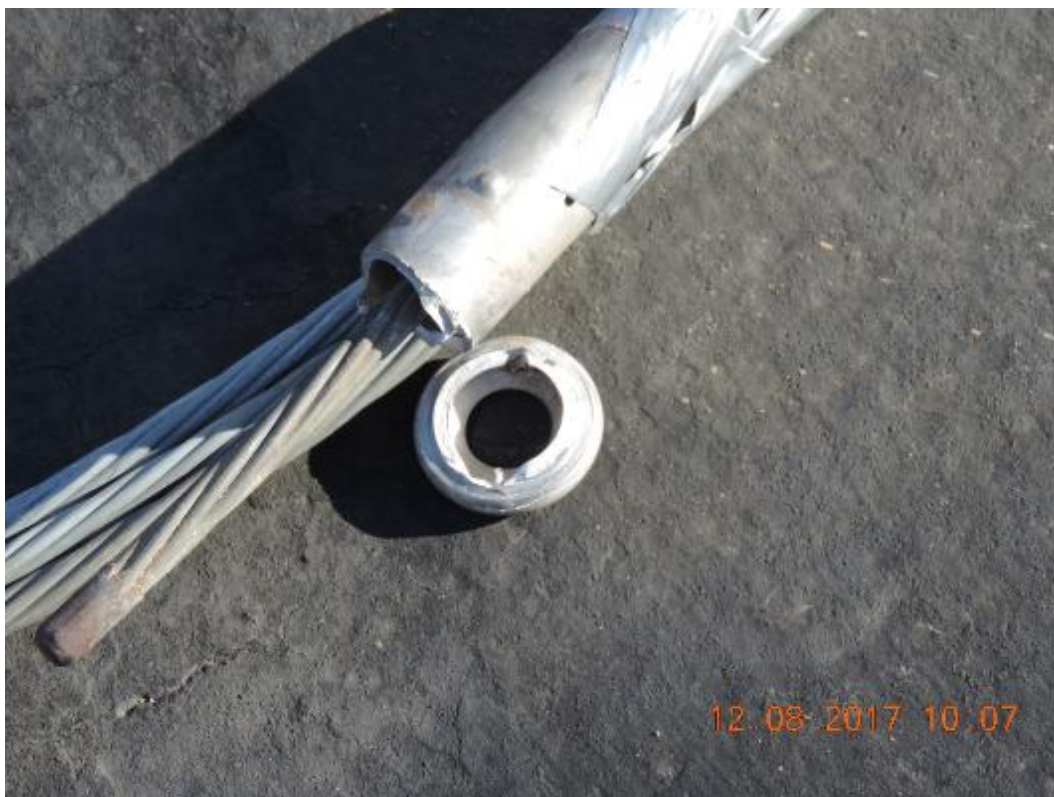
Figure 13: Both pieces of the broken dead end assembly
