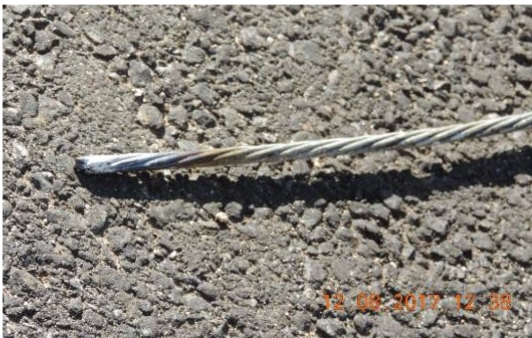
Figure 10: Free end of the approximately 12-foot section of the guy wire found hanging from pole 4389254E
