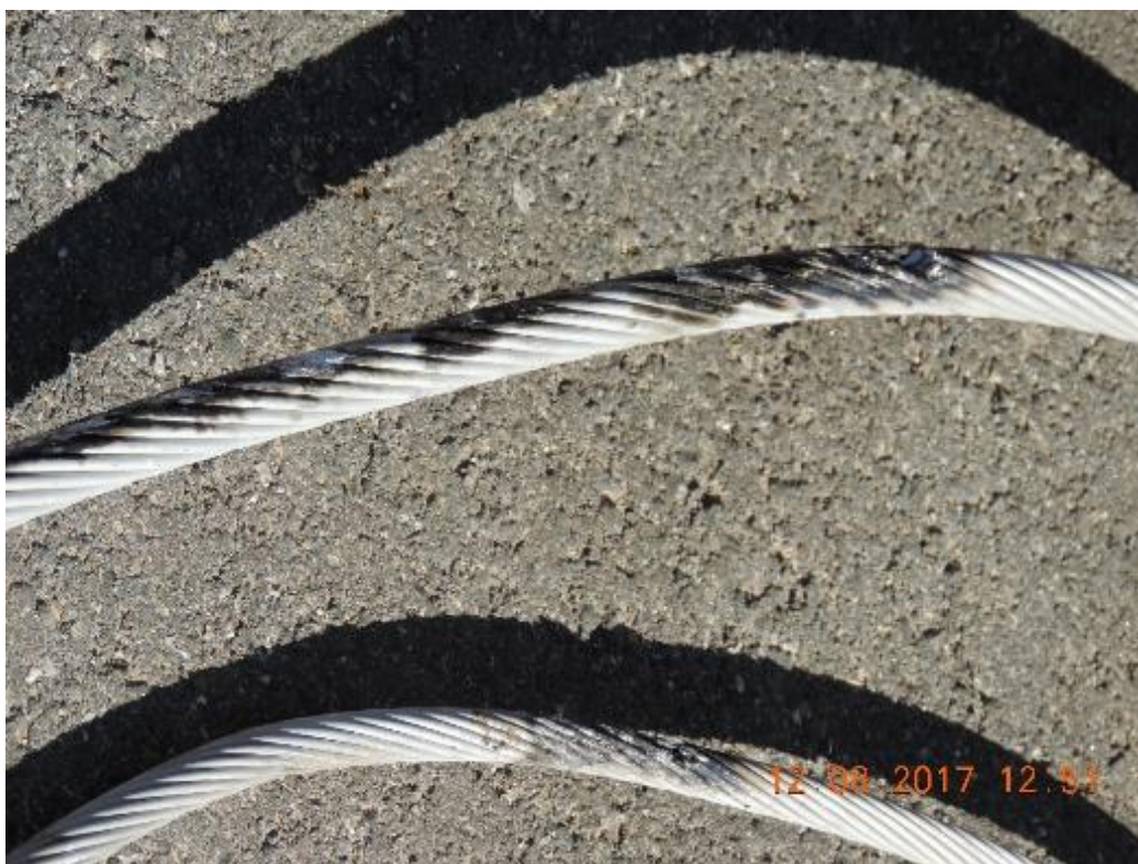
Figure 11: Two jumper wires from pole 4389254E exhibit burns and loss of material.
