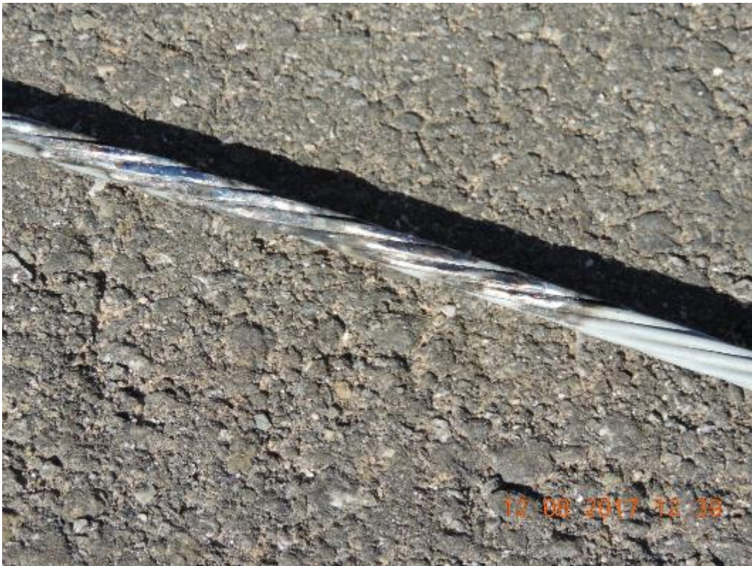
Figure 9: Damage along the approximately 12-foot section of guy wire.
