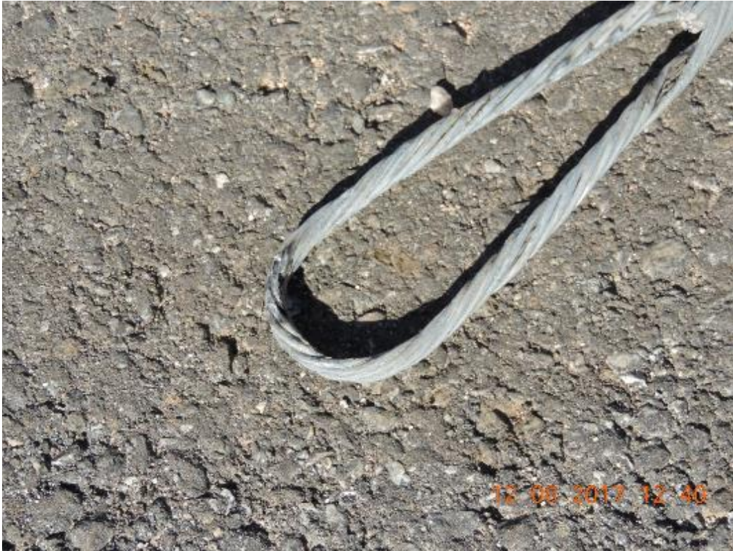
Figure 8: Loop on the approximately 12-foot section of guy wire found hanging from pole 4389254E
