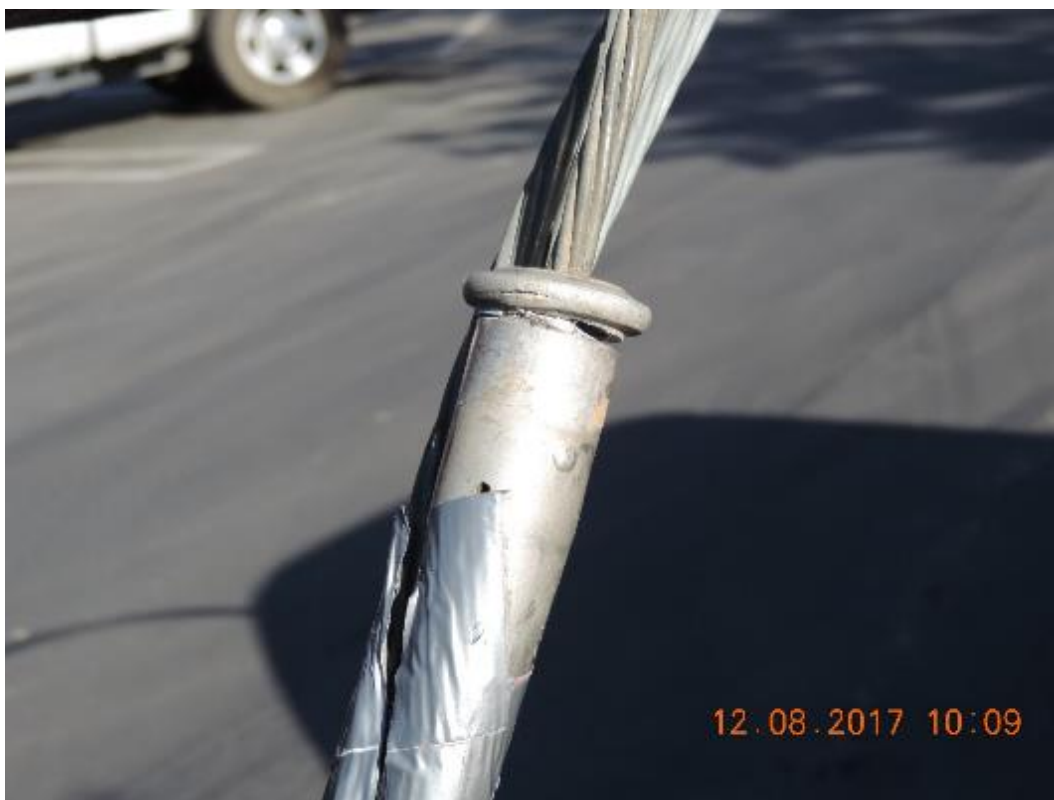
Figure 14: In-service configuration of the two pieces of the broken dead end support.
