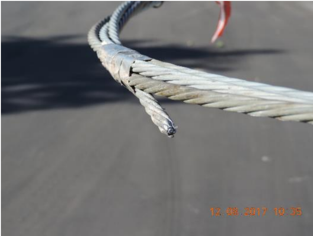
Figure 15: Broken end of 20-foot portion of guy wire
