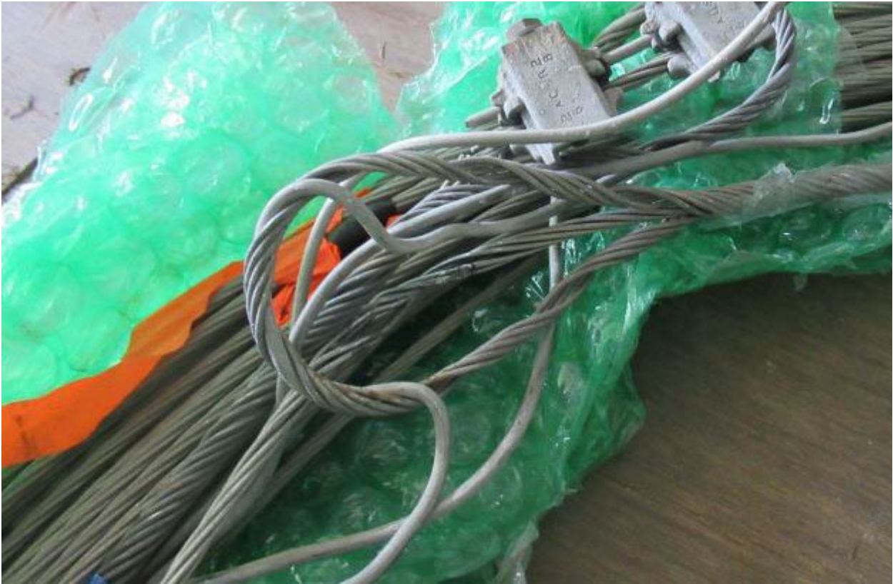
Figure 14: SED photo of February 2017 Anlauf Canyon evidence examination, arc marks and bird-caging on the east conductor between poles numbered 1025341E and 3002114E.
