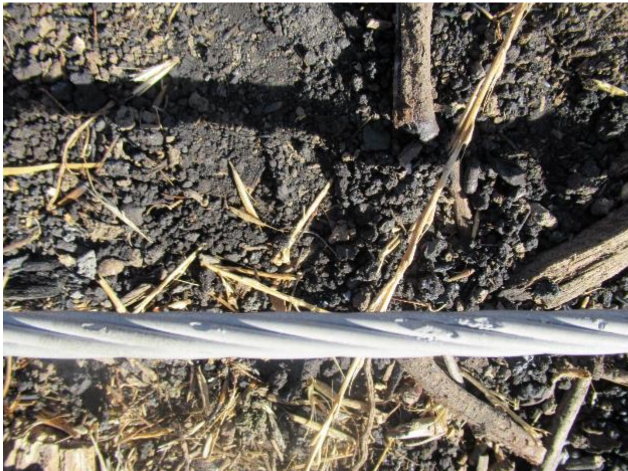
Figure 10: SED photo of Anlauf Canyon site, pitting on the east conductor between poles numbered 3002114E and 1202085E.
