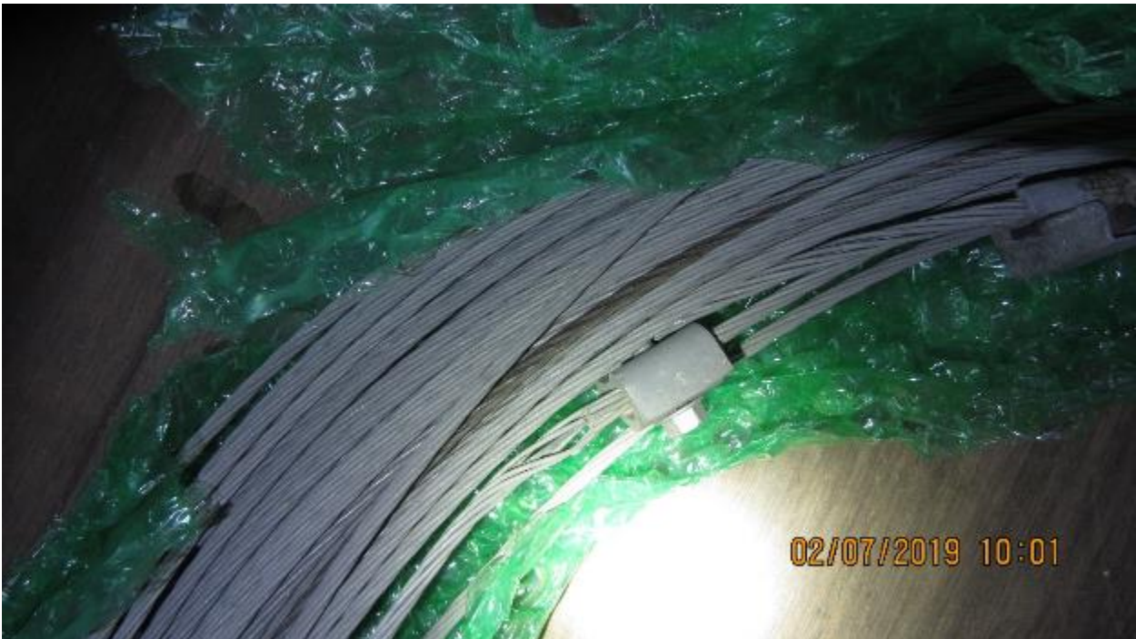
Figure 15: SED photo of February 2017 Anlauf Canyon evidence examination, burn marks and broken strands on center conductor between poles numbered 1025341E and 3002114E.
