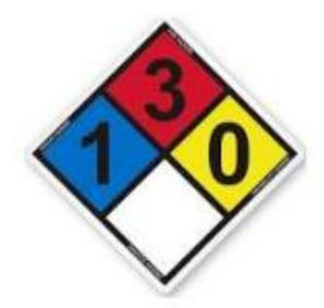
Figure 10: A typical NFPA 704 hazmat placard.
