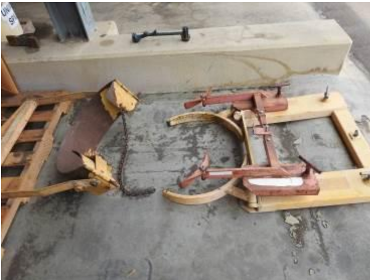
Chemical drum holders at the entrance of the chemical storage room
