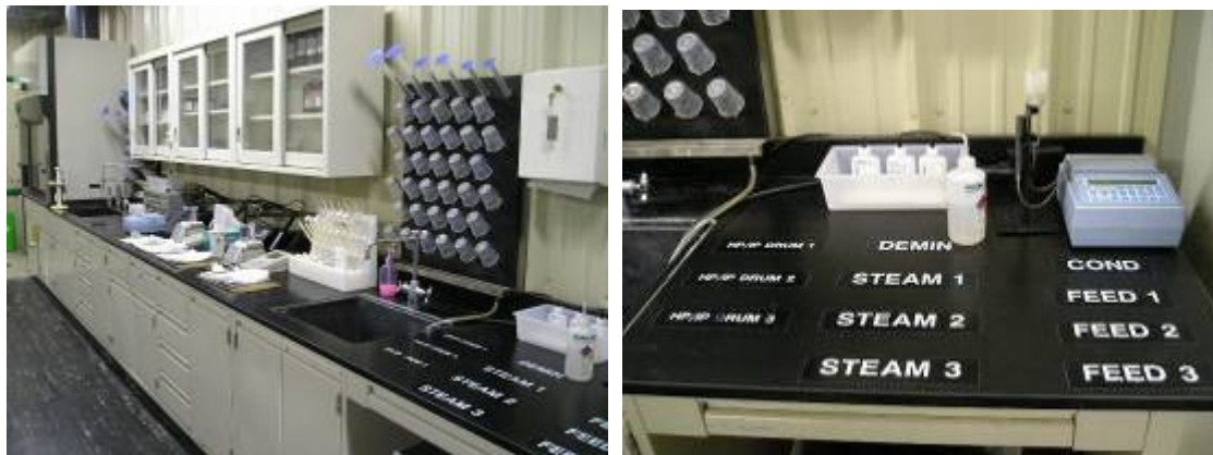
Photo 23: The chemistry analysis table holds multiple water analysis devices and is well organized.
