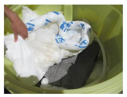
Figure 7: Wet and defective absorbent socks in the spill kit.
