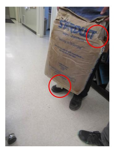
Figure 8: A bag of absorbent had holes causing loose absorbent materials to leak.
