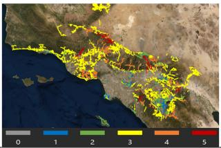
Figure IV-2 - Image showing the Fire Behavior Index levels by circuit.
