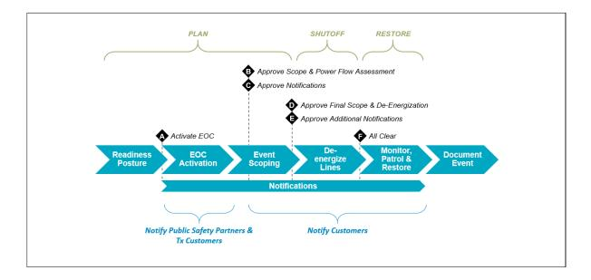
Figure 3: PG&E's High-level PSPS Process Steps
