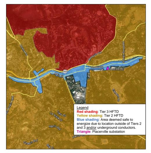
Figure 12: Placerville temporary microgrid
