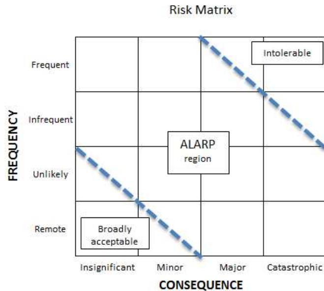
Figure 3: Risk matrix with ALARP labels overlay
