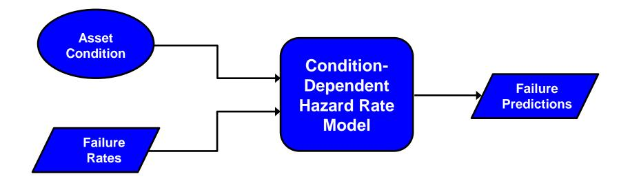
The **Condition-Dependent Hazard Rate Model** specifies failure probability for an asset, given its condition and the occurrence of events that affect failure
