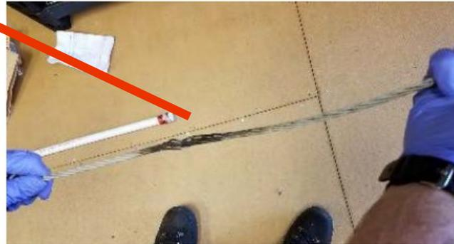
Figure 17: Neutral Conductor
