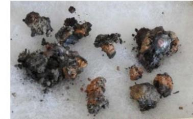
**Figure 12.** Fulgurite-like masses found in the Atlas 1 incident area. CAL FIRE Evidence Log items 5A through 5C.
