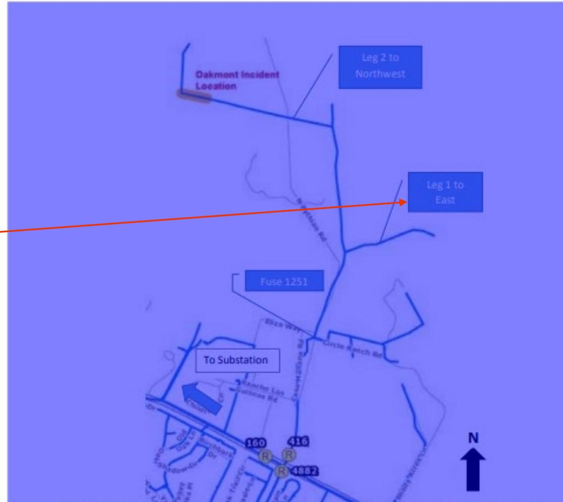
Figure 7. Map of incident location showing approximate locations of upstream reclosers and fuse 1251. (Source: PG&E<sup>22</sup>)
