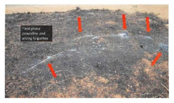
Figure 12: Conductor and fulgurites between Pole #10525757 and Pole #05172 (Source: CAL FIRE)
