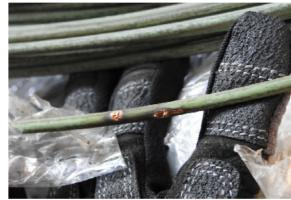
Figure 14. Beading on the subject copper span in the Atlas 2 incident area. CAL FIRE evidence item 3A.
