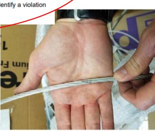
Figure 11. West conductor with burn mark.
