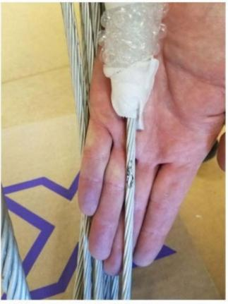
Figure 10. East conductor with burn mark.
