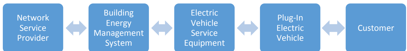
Figure 1: Entities included within the provision of electricity or information during a charging event.
