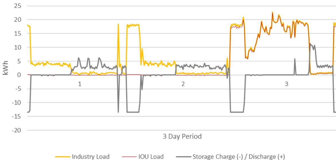
Storage systems inherently increase energy consumption. Because of losses in the battery, less energy can be discharged than is stored in the battery. This fact provided an additional QC benefit. After we removed data that were completely missing or clearly corrupt, we examined the roundtrip efficiency (RTE)
