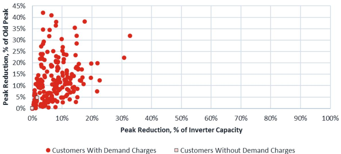
Two customers under the same rate schedule can differ dramatically in their abilities to reduce peak demand if, say, one customer has a low, flat load profile for most of the day with a dramatic one-hour spike, whereas the other has a flat, but high-demand, load profile. While the goal of demand charges is to minimize the need for generation capacity, they are not always effective at reducing demand in peak
