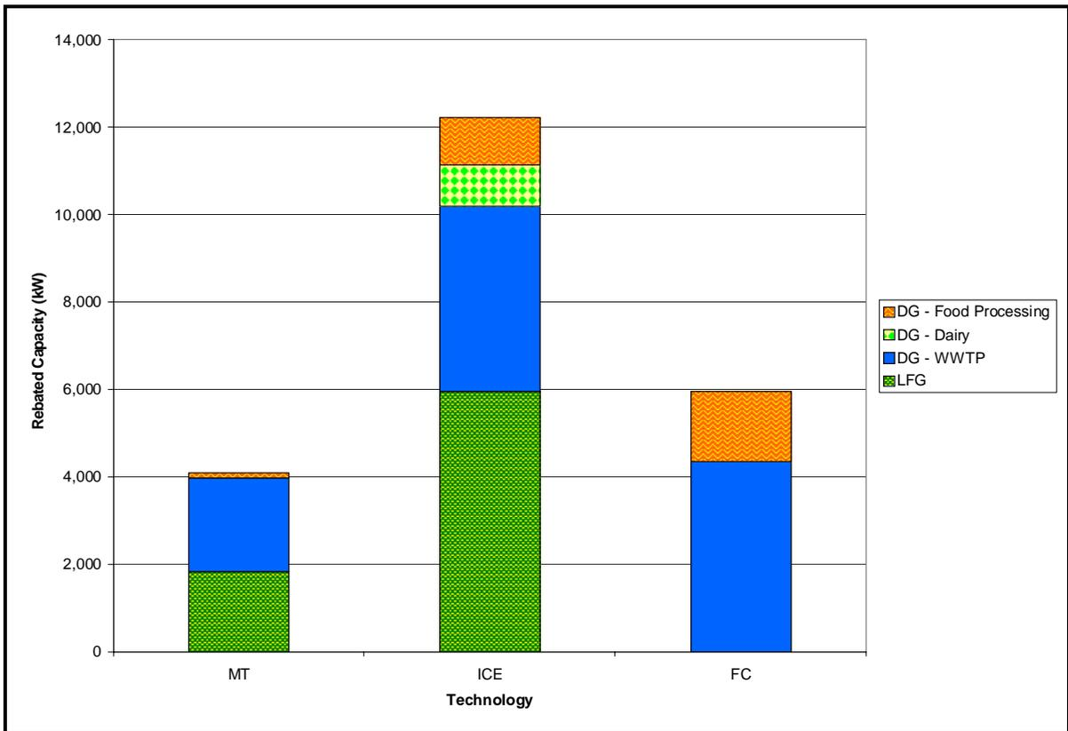
LFG = landfill gas; WWTP = wastewater treatment plants; MT = microturbines; ICE = IC engines; FC = fuel cells; DG= digester gas
