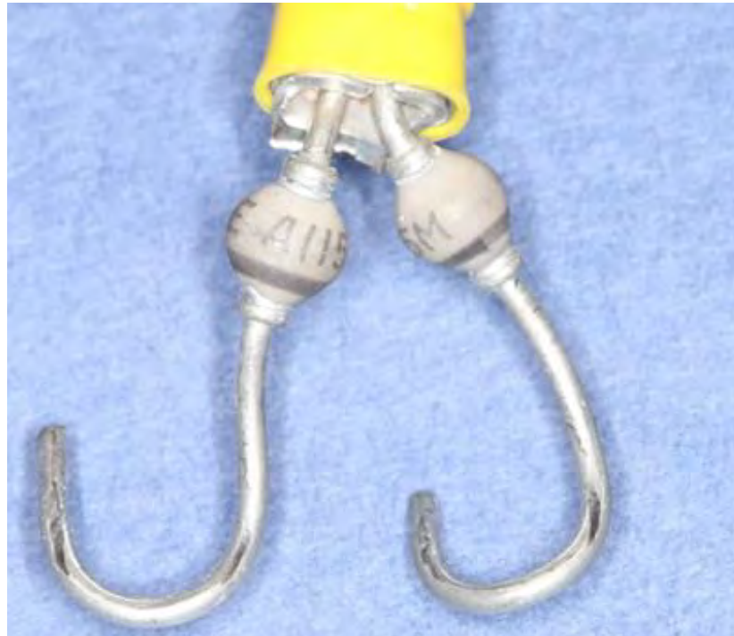
Figure 4. The 600V fast recovery diodes after disconnecting from the incident switch terminals.
