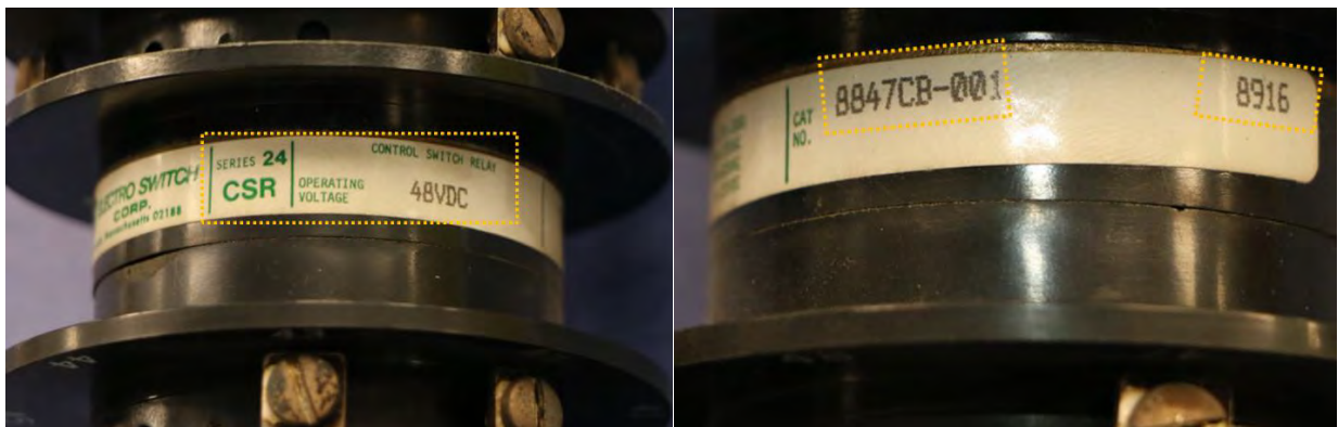
Figure 2. Incident switch markings: CSR 24, 48 VDC, catalogue No. 8847CB-001, serial No. 8916.
