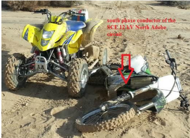
Figure 3. The south phase conductor of the SCE 12 kV North Adobe circuit was found on top of a motorcycle.
