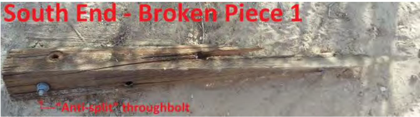
Figure A-3: "South End – Broken Piece 1" (photo 1/4) is the larger of the two pieces that broke off from the South End.
