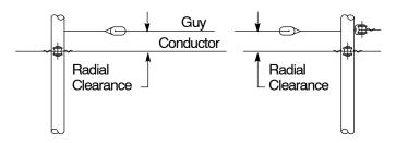
Figure 10 Radial Clearance (see Note 1)
