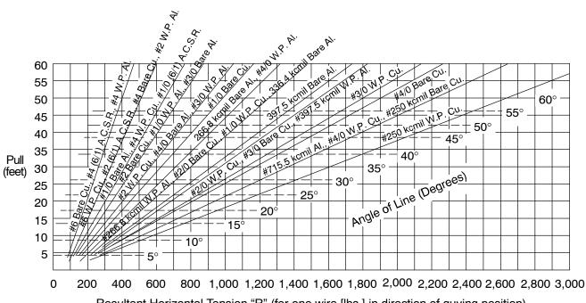
Resultant Horizontal Tension "R" (for one wire [lbs.] in direction of guying position)
