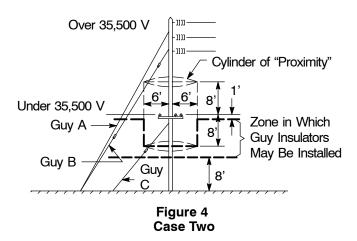
Guy A is not in proximity to supply conductors of 0–35,500 V and is not exposed. Since Guy A is not in proximity and is not exposed, there is no requirement to add sectionalizing. (Note: Guy A may be sectionalized if required by permitting agency.)
