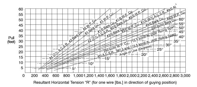
Figure 40 Resultant Tension "R," Heavy or Intermediate Loading
