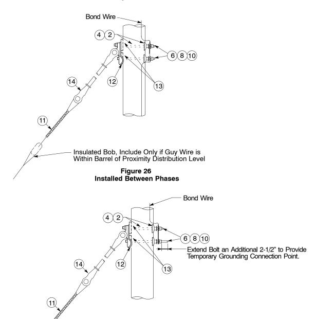
Figure 27 Installed Below Circuit
