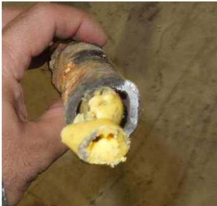
Figure 5: The service riser inserted with plastic.
