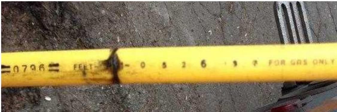
Figure 6: Date stamp on inserted plastic for service of [REDACTED] indicating 052697.
