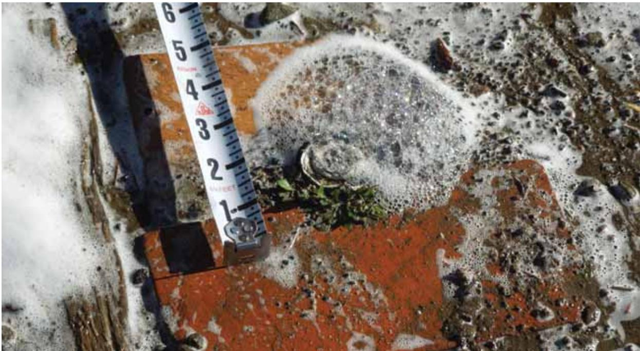
**Figure 8.** Air bubbles around a sprinkler head
