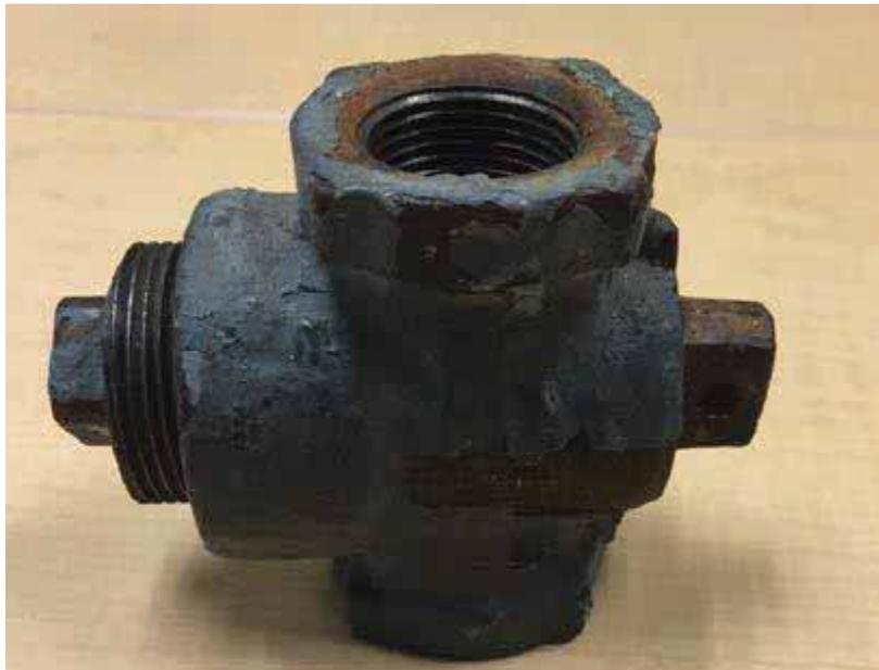
*Figure 9: A typical Nordstrom valve. The packing nut is on the left of the valve body, and the tang is to the right. The tang of the valve at [REDACTED] had been broken off, and the valve was inoperable.*
