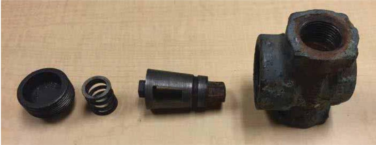
*Figure 10: The various parts of a typical Nordstrom valve, from left to right: packing nut, spring, valve core (with tang on the right-hand side), and valve body. When the nut, spring, and core are removed, there are 2 openings on the sides of the valve body that gas can flow out from.*
